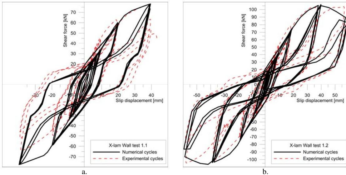
**Figure 4.3.** Numerical-experimental comparison on cyclic behaviour of X-Lam panel 1.1 (left, a.) and panel 1.2 (right b.)
