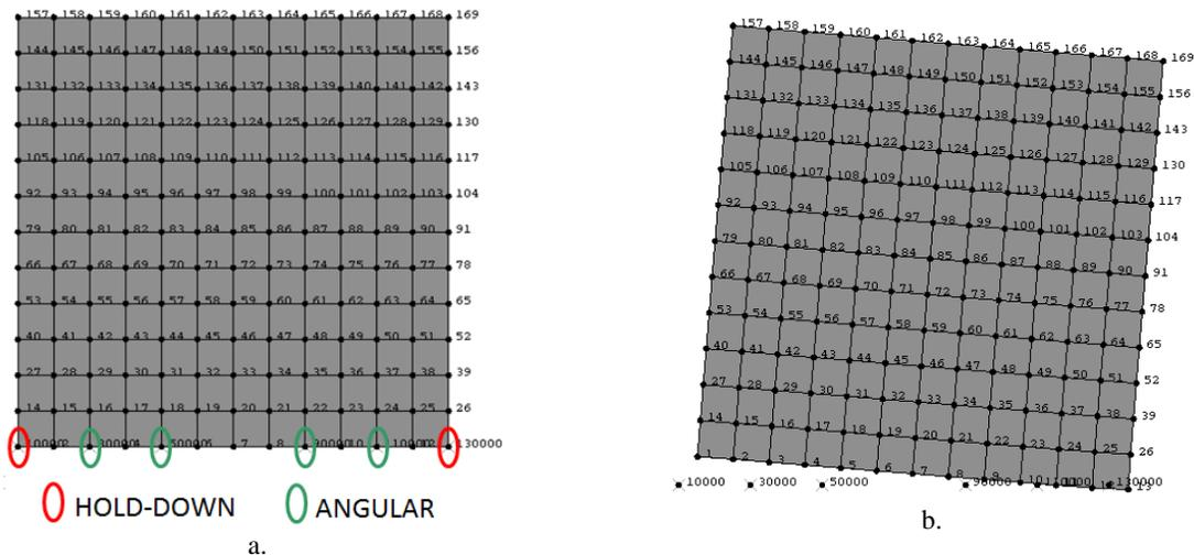
**Figure 4.2.** Mesh and springs used to model the Panel 1.2. (left ,a.) and an example of deformed shape predicted in the numerical analysis (right, b.)
