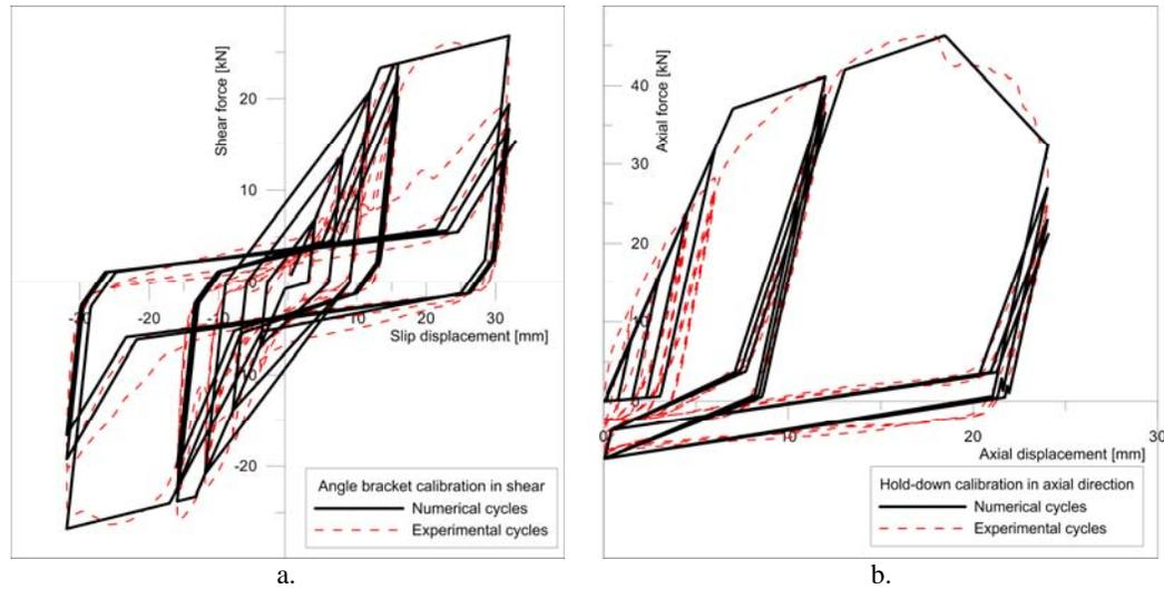
**Figure 4.1.** Calibration of angle bracket springs (left, a.) and calibration of hold-down springs (right, b.)
