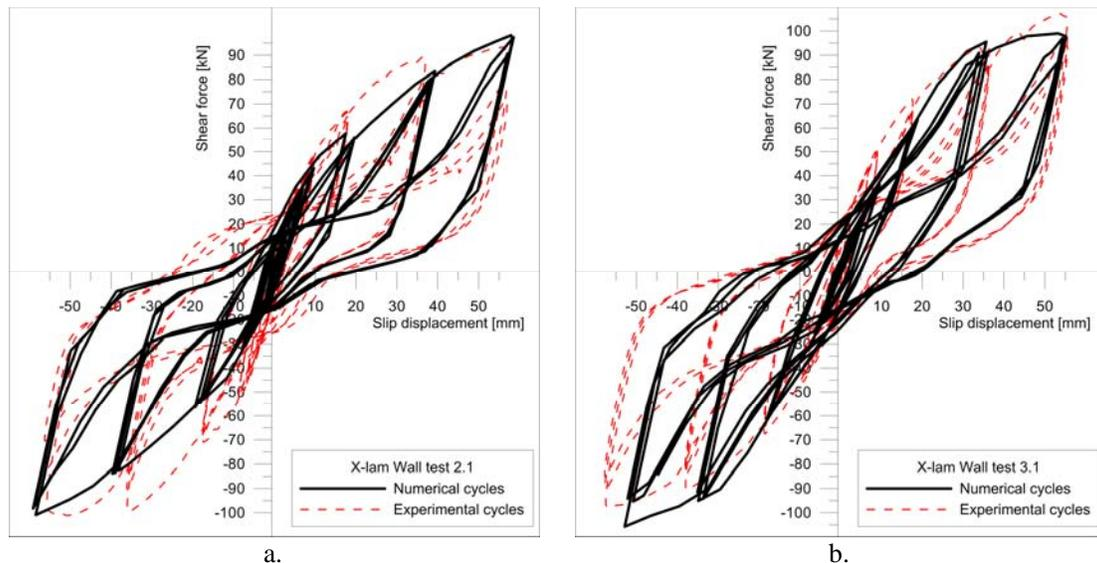
**Figure 4.4.** Numerical-experimental comparison on cyclic behaviour of X-Lam panel 2.1 (left, a.) and 3.1 (right, b.)
