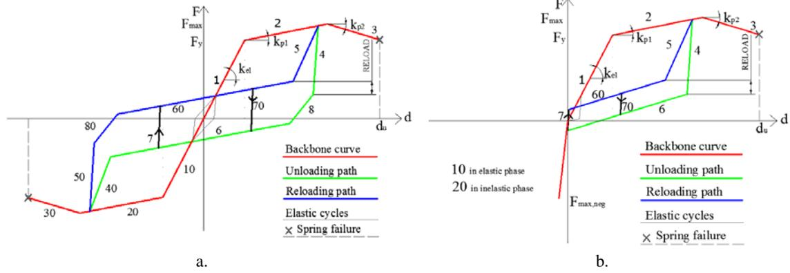
**Figure 2.1.** Piecewise linear relationship of screws and angle bracket springs (left, a.) and hold-down springs (right, b.)
