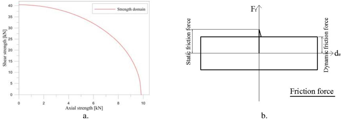
**Figure 2.2.** Strength domain (left, a.) and friction force at constant axial load (right, b.)
