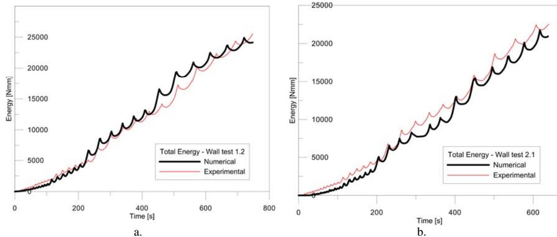
**Figure 4.5.** Numerical-experimental comparison of time-history of the total dissipated energy during the cyclic tests on X-Lam panel 1.2 (left, a.) and 2.1 (right, b.)
