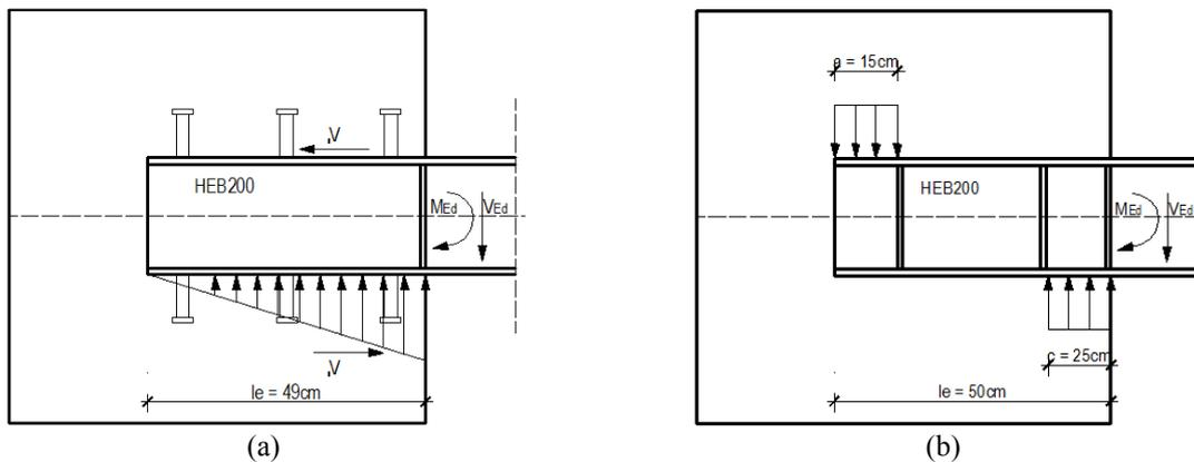
**Figure 5.** Connection typology 1 (a) and typology 2 (b).
