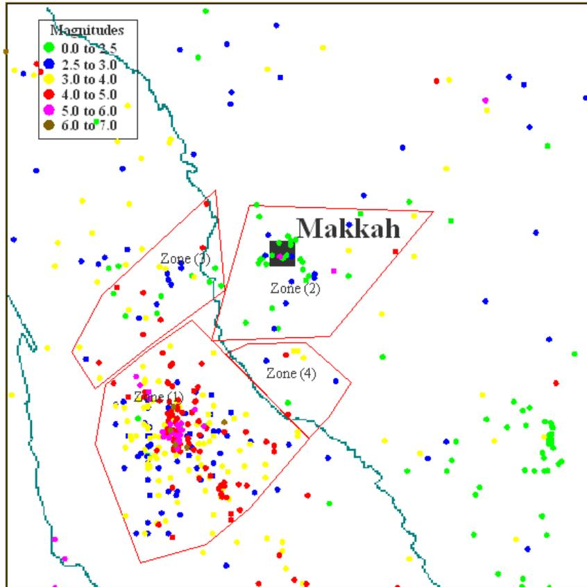
**Figure 5.** Seismic source zones for deterministic study
