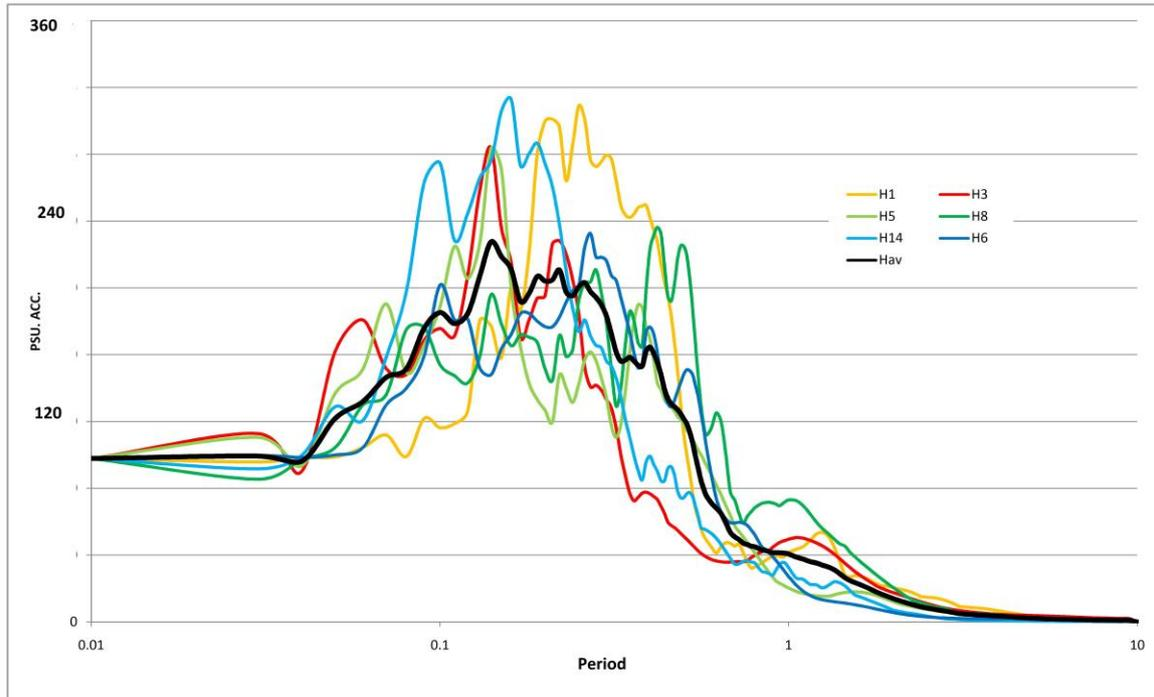
**Figure 7.** Response spectra for the selected earthquakes
