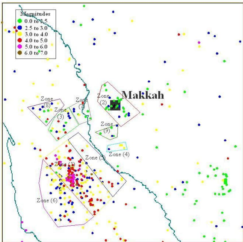
**Figure 6.** Seismic source zones for probabilistic study
