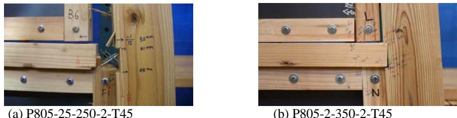
Figure 3.2. Failures of Connections at Drift Angle  $-1/15\text{rad}$ .
