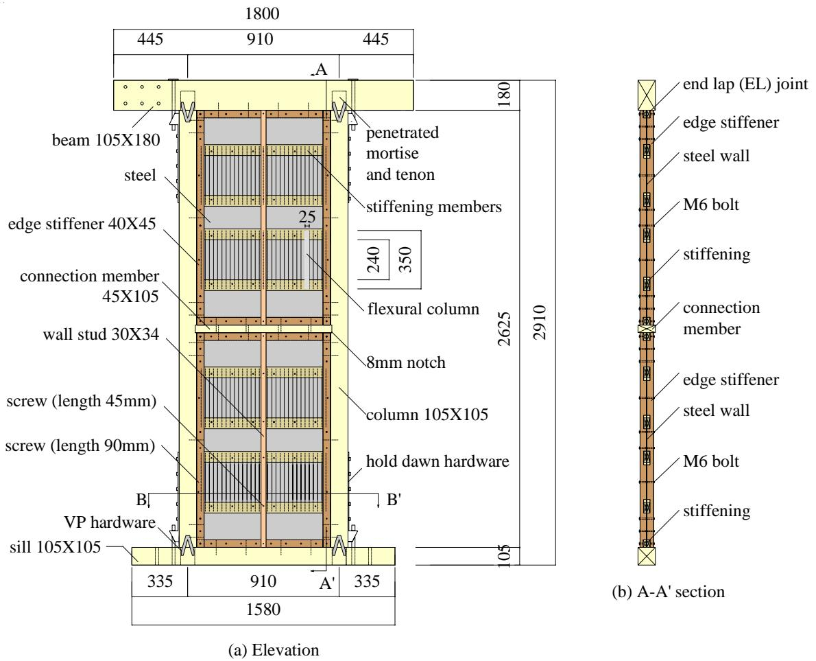
**Figure 2.1.** Details of specimen P805-25-350-2-T45
