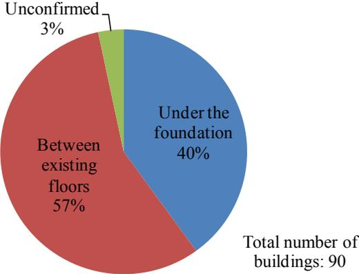
Figure 2.3.2. Ratio of the location of seismic isolation layer
