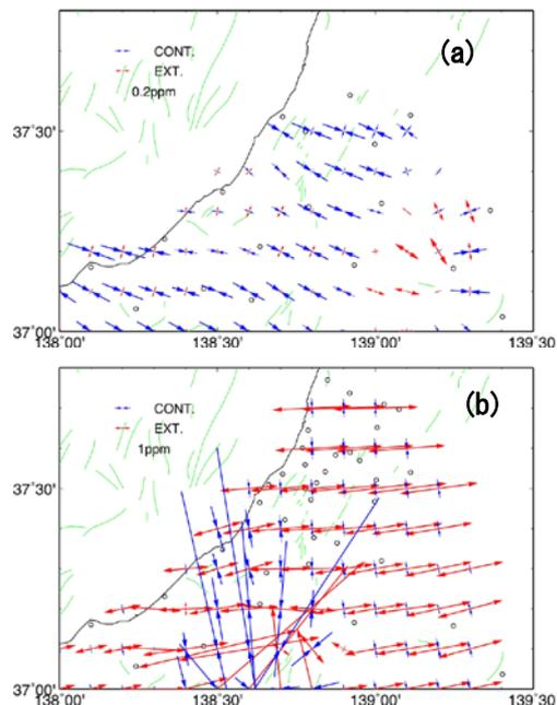
**Figure 4.** Principal strain axes distribution (a): before the earthquake (2009/01-2011/01, GEONET) (b): on the earthquake (AN-net and GEONET)
