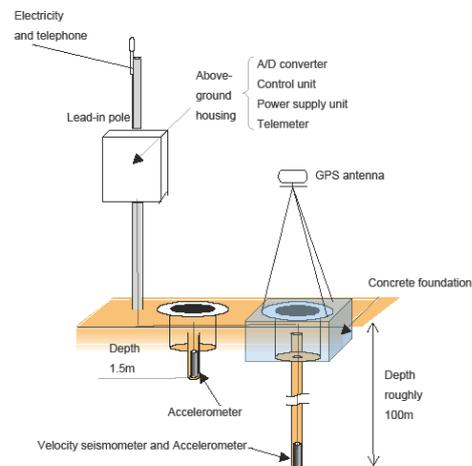
**Figure 2.** Configuration of the AN-net station
