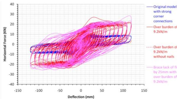
**Figure 21.** Hysteresis loop comparisons at 9.2kN/m
