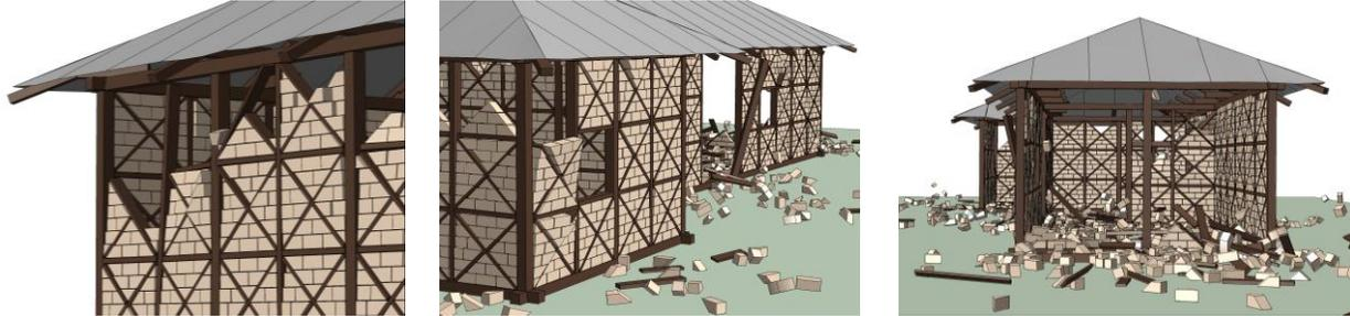
**Figure 9.** Close up of building behaviour without nails.
