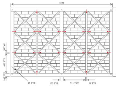
**Figure 12.** Wall panel push over model
