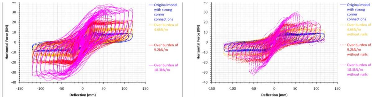
**Figure 18.** Hysteresis loops of varying levels of overburden with and without nails.
