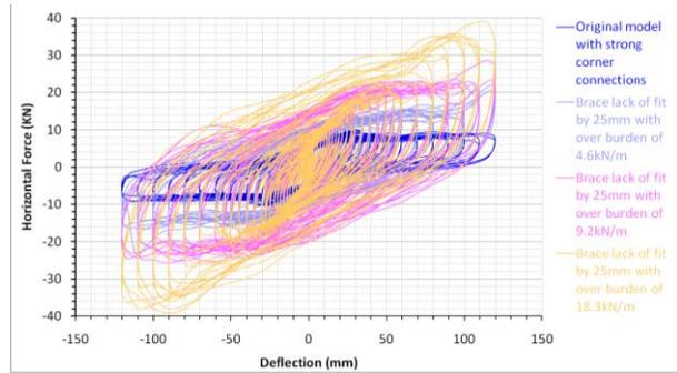
**Figure 20.** Hysteresis loops of increased overburden and brace shortening
