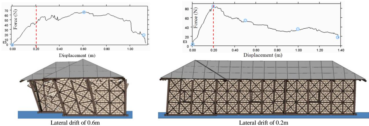
**Figure 10.** Force deflection curves and images of the two orthogonal building directions [with nails]
