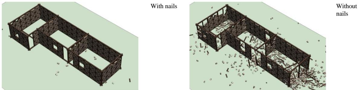
Figure 8. Final building condition after earthquake time histories (roof not shown for clarity)
