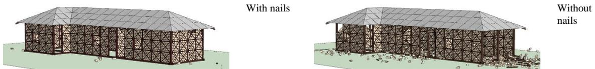
Figure 7. Final building condition after earthquake time histories
