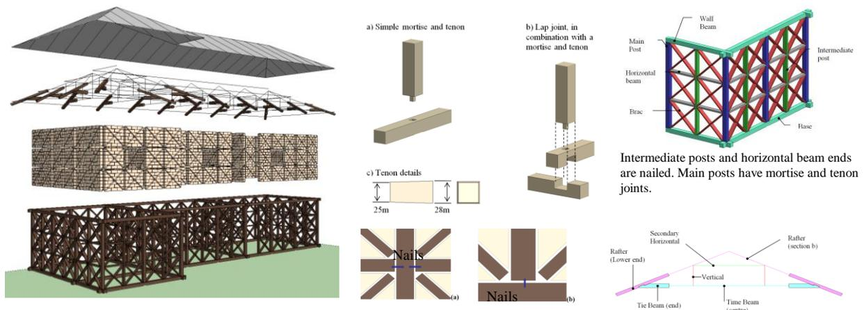
**Figure 3.** Exploded view of full *dhajji dewari* model and model details
