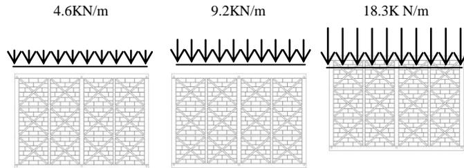
**Figure 16.** Three levels of overburden.
