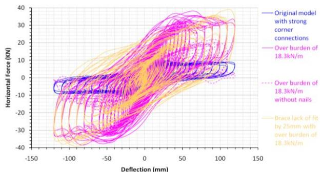
**Figure 22.** Hysteresis loop comparisons at 18.3kN/m
