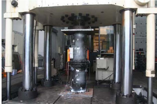
**Figure 5.** The 500-ton universal testing machine in joint compression tests
