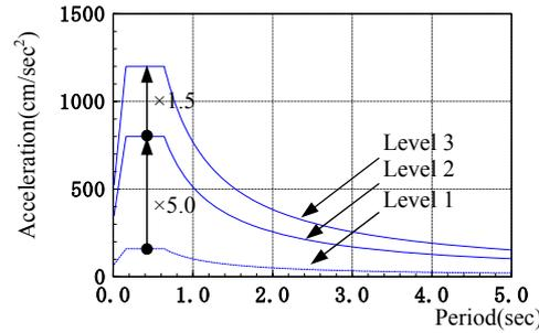
**Figure 2.** Acceleration spectrum of input earthquakes( $h=5\%$ )
