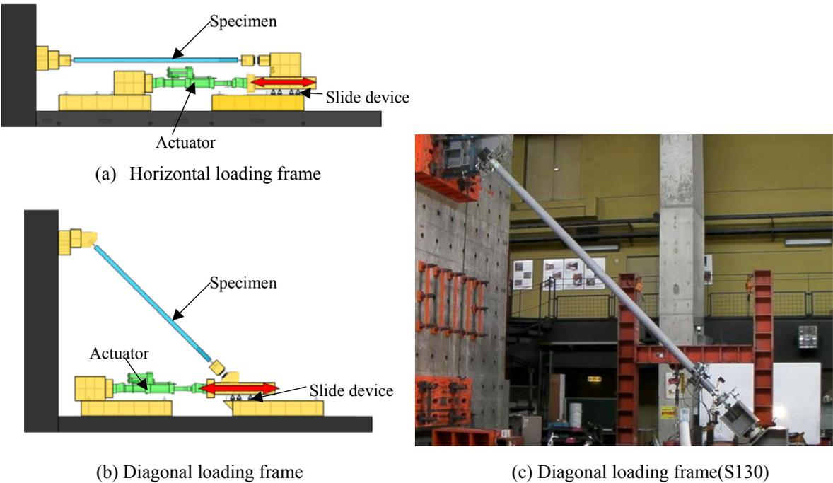
**Figure 12.** Configuration of loading frame
