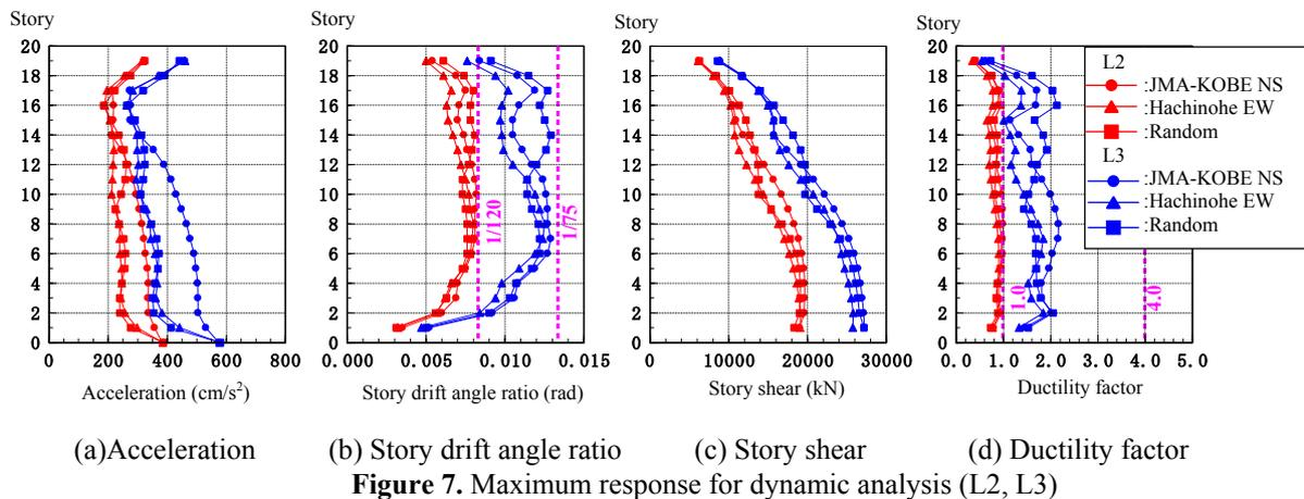
Figure 7. Maximum response for dynamic analysis (L2, L3)
