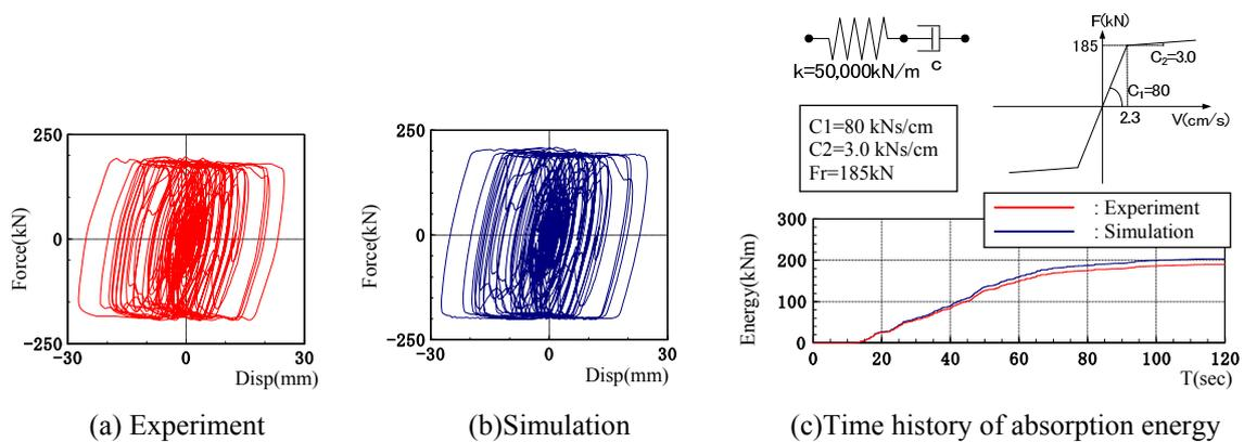
Figure 15. Force-displacement relation under Random Loading (L140)
