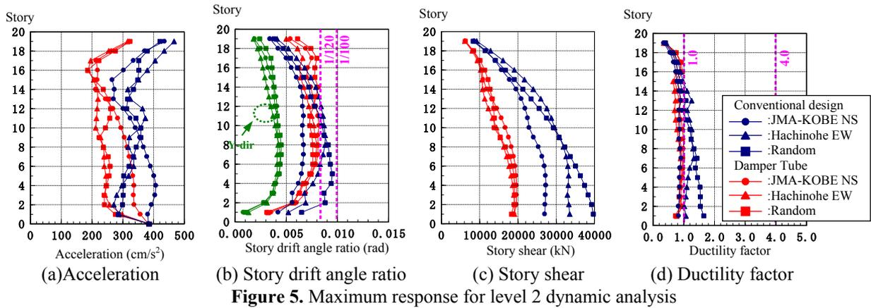
Figure 5. Maximum response for level 2 dynamic analysis
