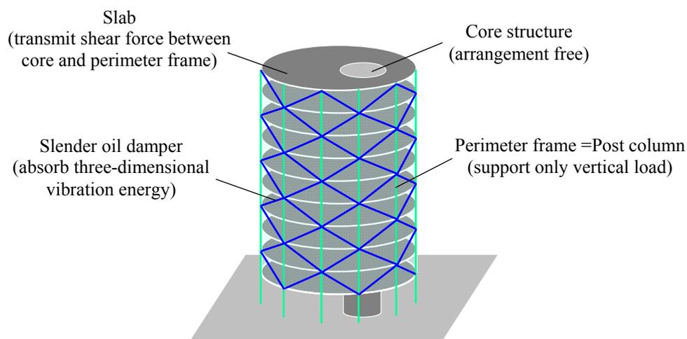
Figure 1. Conceptual diagram of Damper Tube Structure
