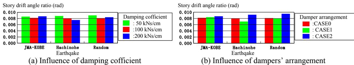
Figure 9. Maximum response for level2 dynamic analysis
