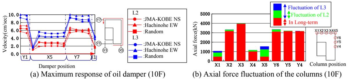
Figure 8. Maximum response for dynamic analysis (L2, L3)
