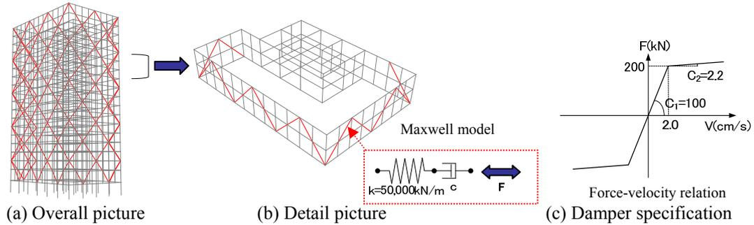
**Figure 4.** Analytical model (DTS)
