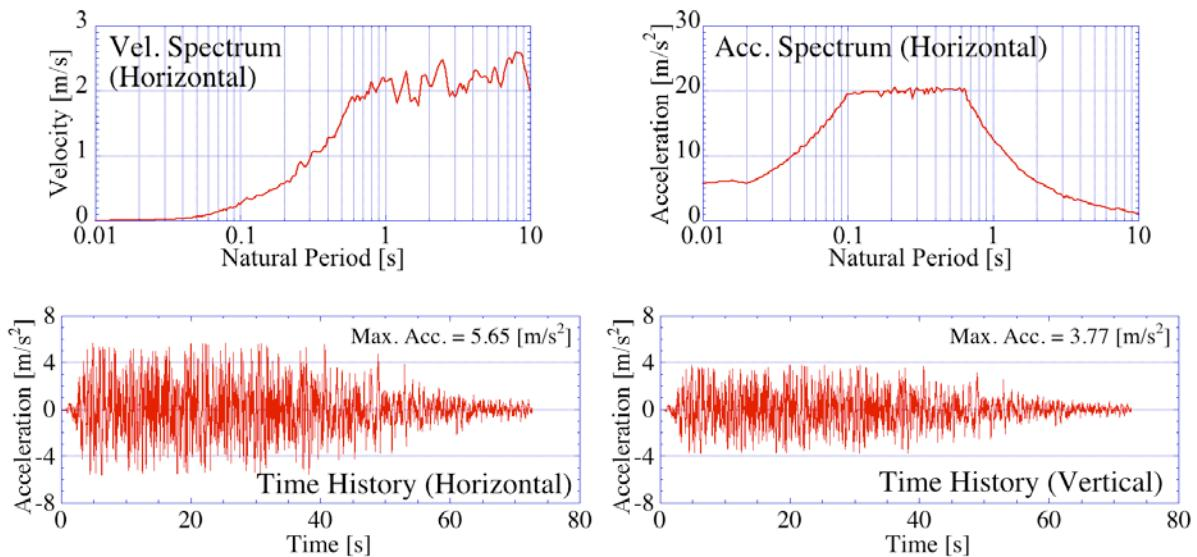
**Figure 6.** Characteristics of input waves
