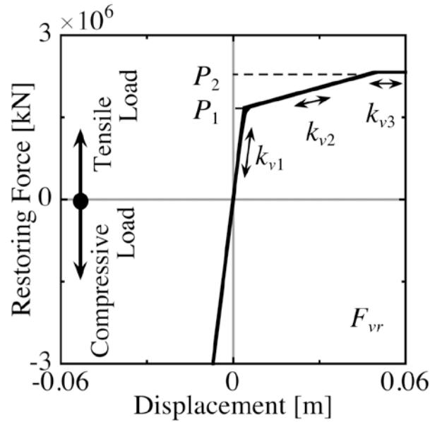
**Figure 4.** Vertical restoring characteristics of rubber bearing
