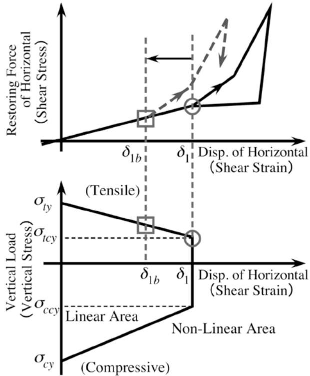
**Figure 5.** Vertical load dependency of hardening starting displacement
