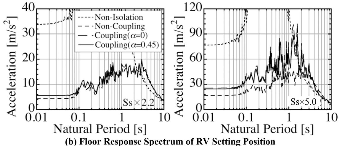
Figure 7. Analytical results of horizontal direction
