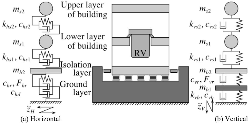
**Figure 2.** Analytical model of building
