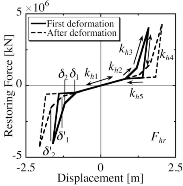
**Figure 3.** Horizontal restoring characteristics of rubber bearing
