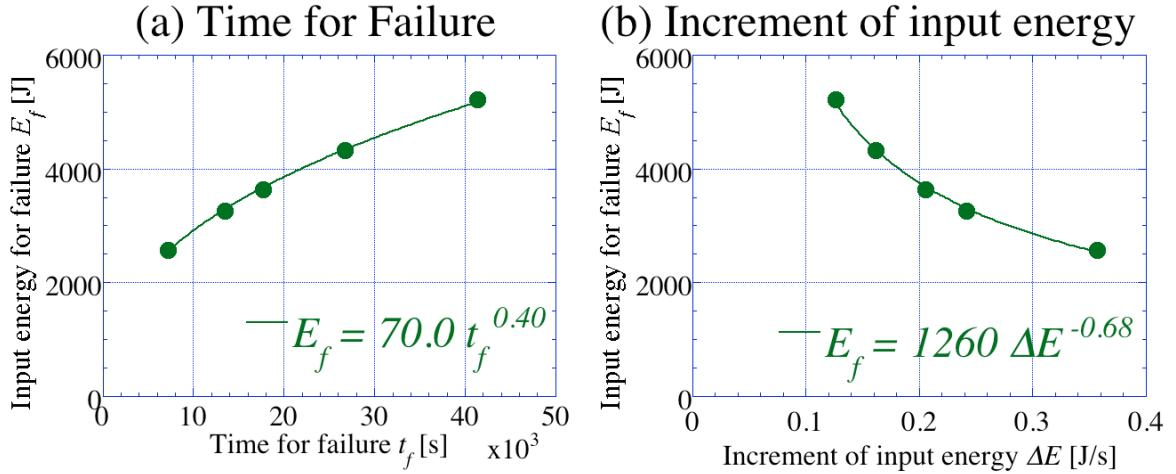
**Figure 3.** Relationships between energy and failure
