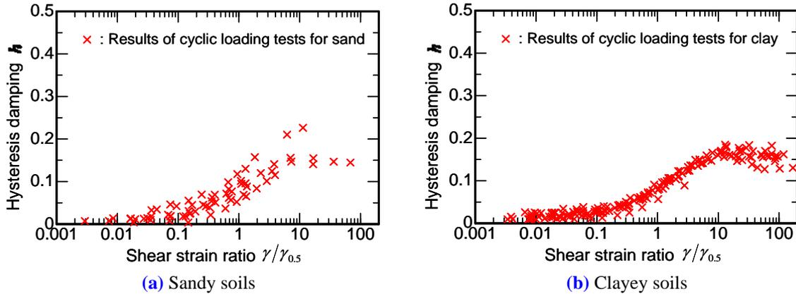
Figure 4.4  $h - \gamma/\gamma_{0.5}$  relationship obtained from cyclic loading tests
