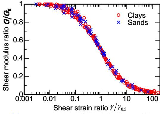
**Figure 4.1**  $G/G_{\max} - \gamma/\gamma_{0.5}$  relationship obtained from cyclic loading tests
