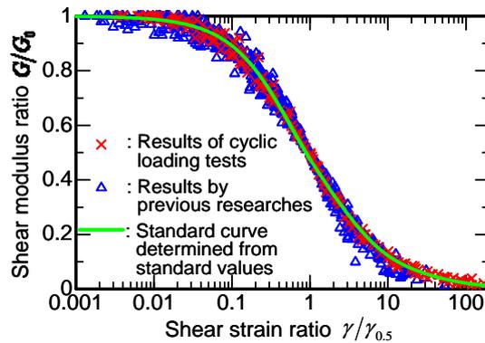
**Figure 4.3**  $G/G_{\max} - \gamma/\gamma_{0.5}$  relationship with “standard curve”
