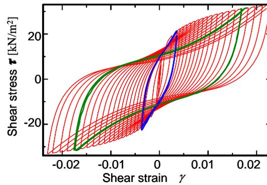
**Figure 3.3** Hysteresis loop of a numerical calculation
