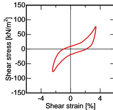
Figure 2.2 Hysteresis loop at large level of strain
