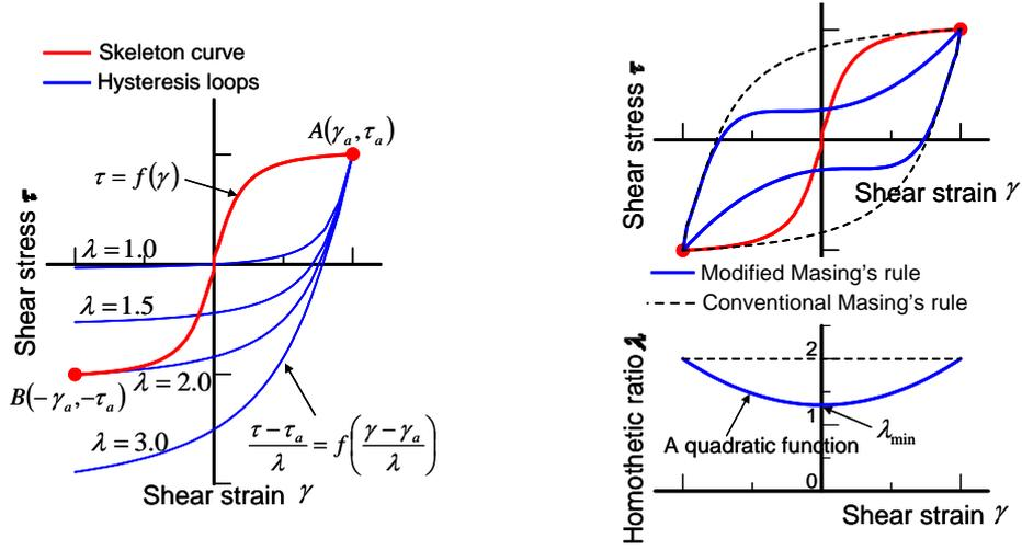
**Figure 3.1** Hysteresis loops with some homothetic ratio **Figure 3.2** Concept of modified Masing's rule (Above: hysteresis loop, below: similarity function)
