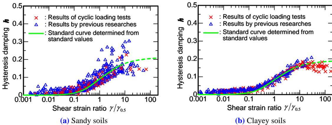
Figure 4.5  $h - \gamma/\gamma_{0.5}$  relationship with “standard curve”
