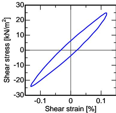
Figure 2.1 Hysteresis loop at small level of strain
