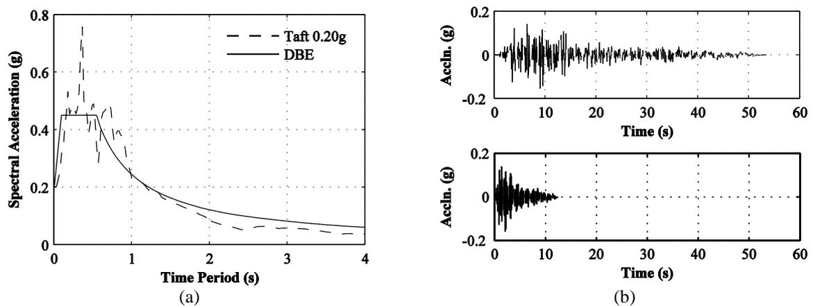
Figure 2.4. (a) Comparison of DBE for Zone V (PGA 0.18g) with Taft (PGA 0.20g) (b) Original and compressed Taft N21E ground motion
