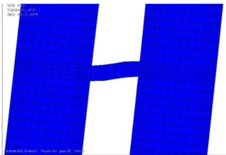
**Figure 4.7.** The deformation of conventional coupling beams
