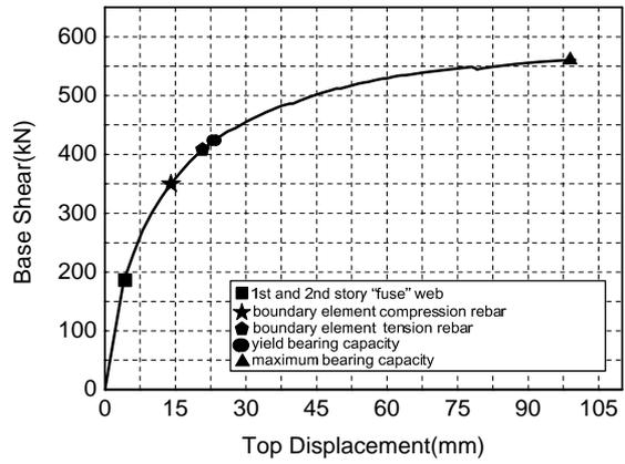
**Figure 4.4.** Base shear-top displacement curves of shear wall with replaceable coupling beams
