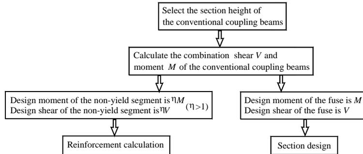
**Figure 2.1.** New coupling beam design flow chart
