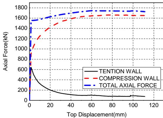
**Figure 4.11.** Axial force-top displacement curves of conventional shear wall
