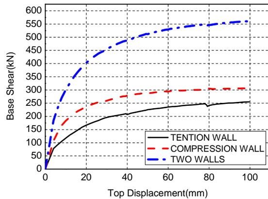
**Figure 4.10.** Base shear-top displacement curves of shear wall with replaceable coupling beams
