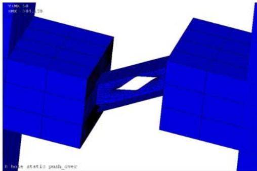
**Figure 4.5.** The deformation of replaceable coupling beams
