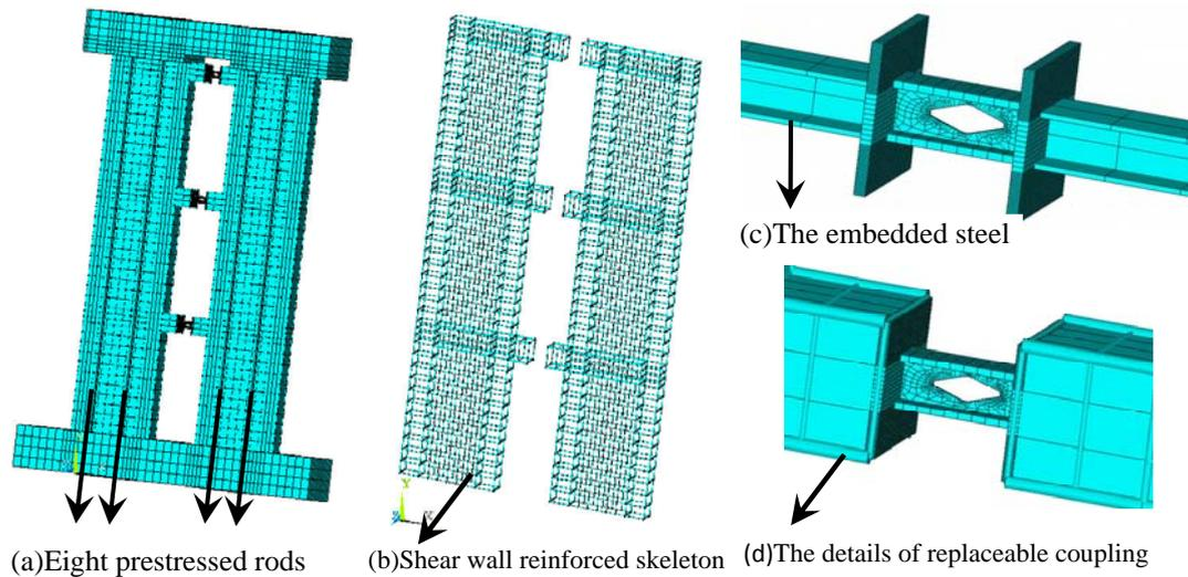
**Figure 4.2.** The shear wall with replaceable coupling beams
