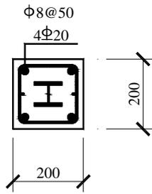
**Figure 3.4.** The reinforcement of non-yield segment
