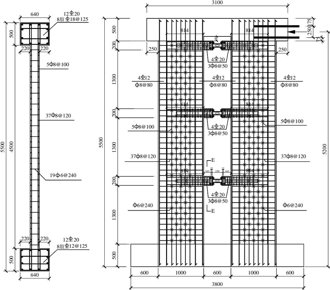
Figure 4.1. Reinforcement of new shear wall with replaceable coupling beams
