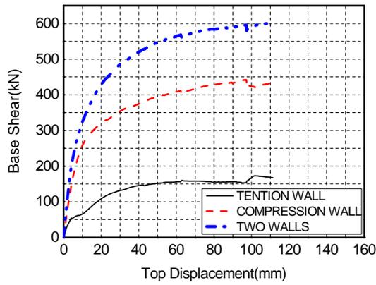
**Figure 4.9.** Base shear-top displacement curves of conventional shear wall
