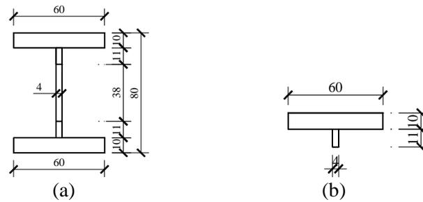
**Figure 3.2.** The cross section in the middle span of “fuse”
