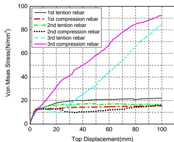
**Figure 4.14.** Von mises stress of longitudinal rebar of replaceable coupling beams
