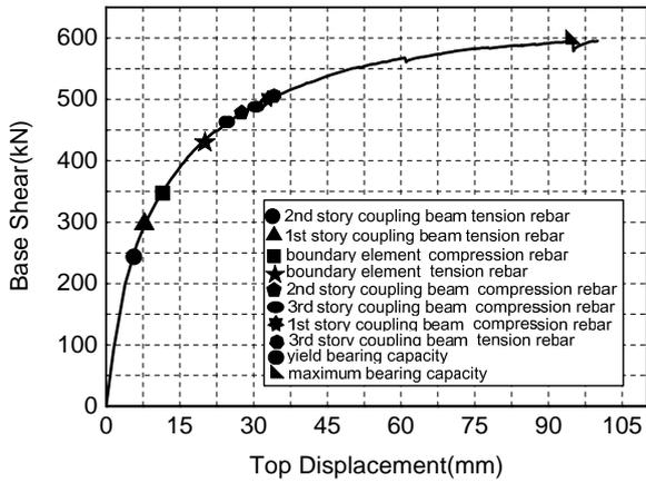
**Figure 4.3.** Base shear-top displacement curves of conventional shear wall
