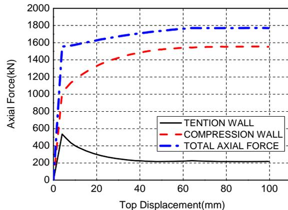
**Figure 4.12.** Axial force-top displacement curves of shear wall with replaceable coupling beams
