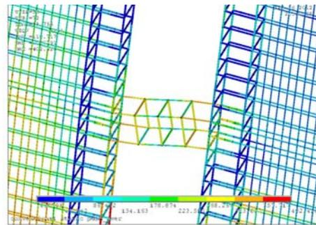
**Figure 4.8.** The von mises of steel rebar of conventional coupling beams
