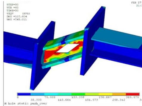
**Figure 4.6.** The von mises of "fuse"
