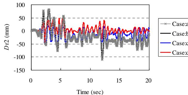
**Figure 3.3.** Time history of relative displacement between right span and transition pier
