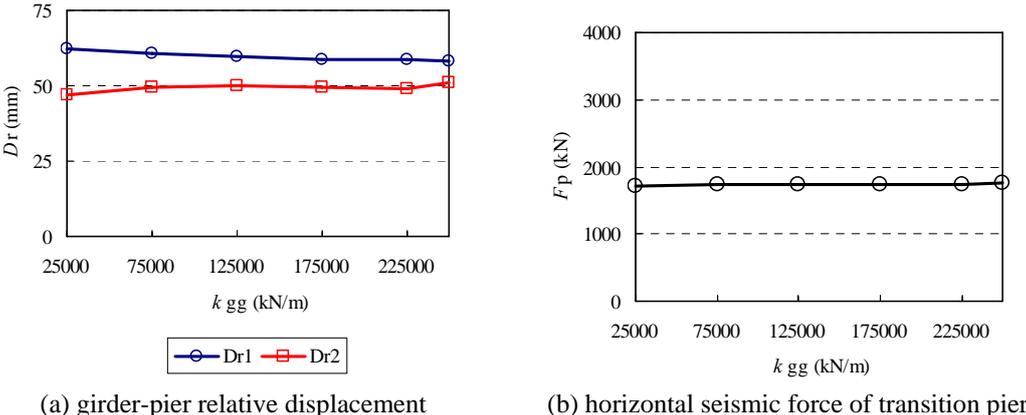
Figure 4.3. Maximum responses of bridge for various stiffnesses of girder-girder restrainer
