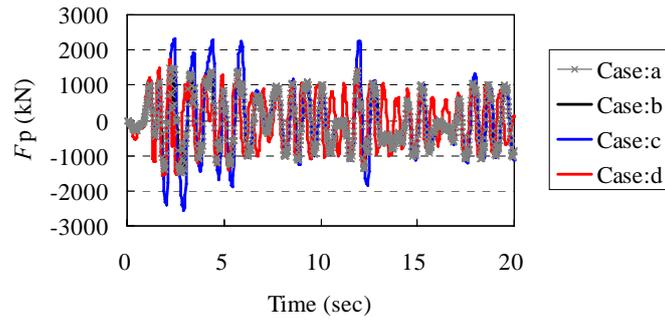
**Figure 3.4.** Time history of horizontal seismic force of transition pier
