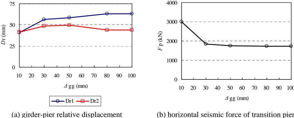
Figure 4.4. Maximum responses of bridge for various gap of girder-girder restrainer
