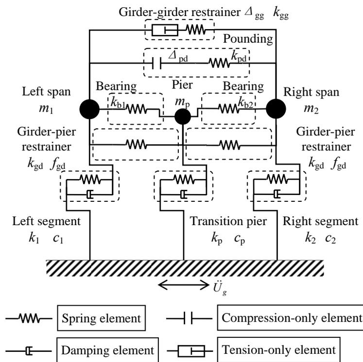
**Figure 3.1.** Simplified mechanical model of multi-level control system of unseating failure
