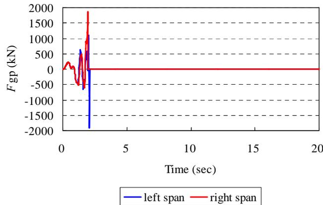
**Figure 3.5.** Time history of control force of girder-pier connection restrainer
