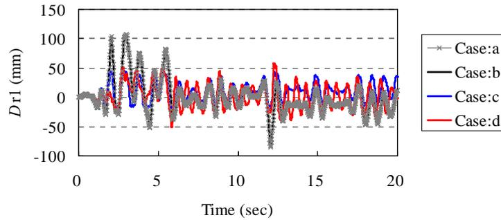
**Figure 3.2.** Time history of relative displacement between left span and transition pier
