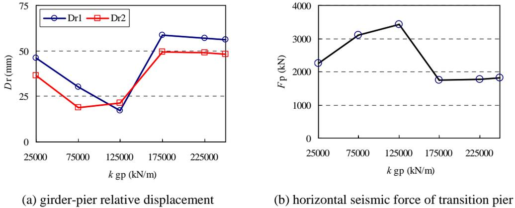
**Figure 4.1.** Maximum responses of bridge for various stiffnesses of girder-pier restrainer
