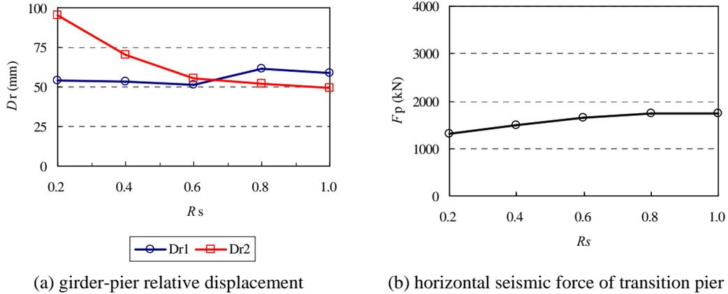
**Figure 4.5.** Maximum responses of bridge for various stiffness ratio of adjacent spans
