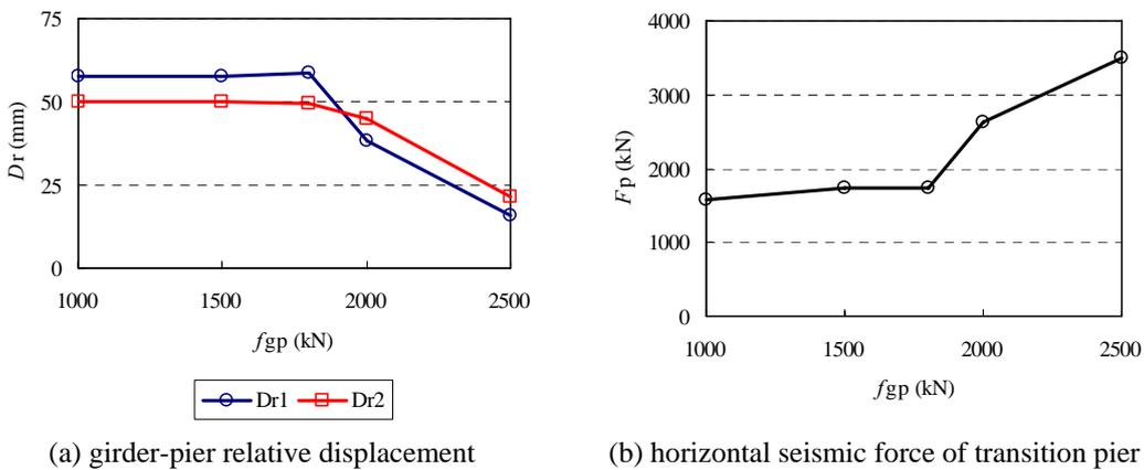
**Figure 4.2.** Maximum responses of bridge for various strength valve value of girder-pier restrainer
