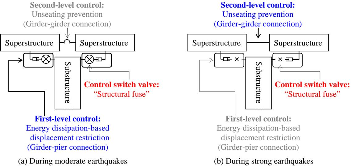
**Figure 2.1.** Illustration of working mechanism of multi-level control system of unseating failure
