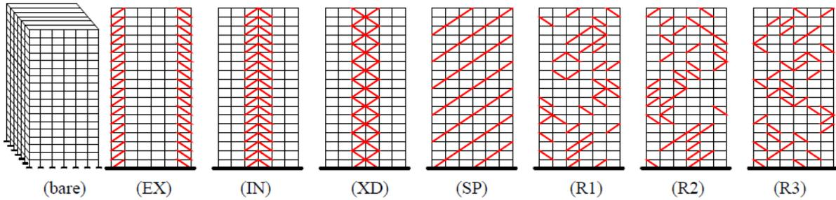
**Figure 2.** Tested Bracing Arrangements of the Perimeter Concrete Frame (Mezzi 2010)
