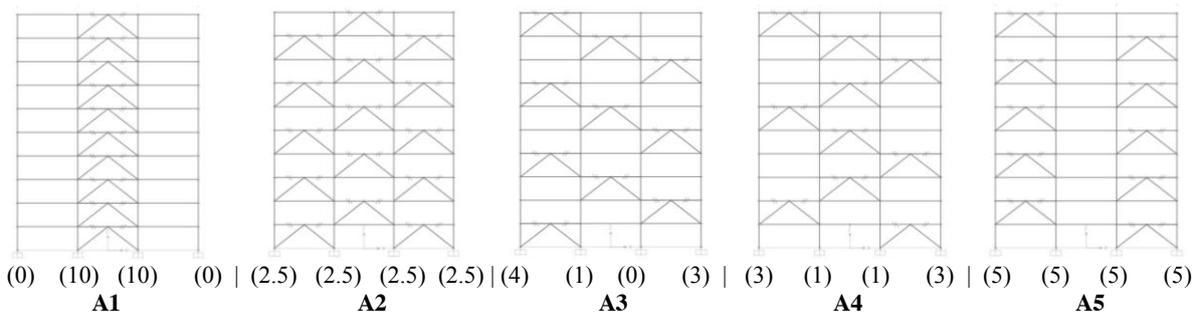
**Figure 3.** Brace-damper Arrangements
