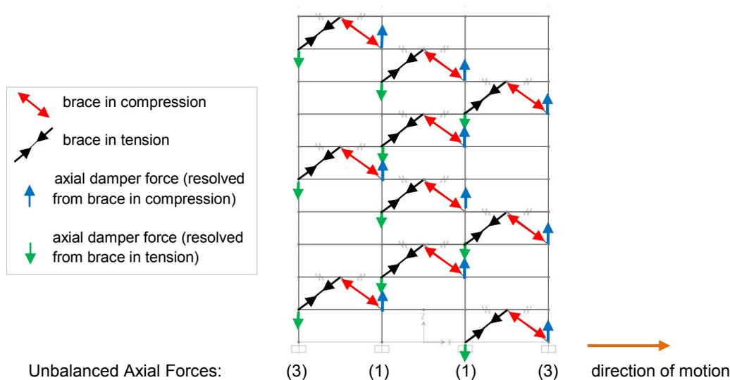
**Figure 4.** Axial Force Counteraction –Unbalanced Damper Reaction Axial Forces for A4
