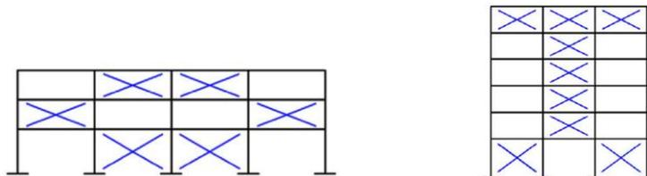
**Figure 1.** Optimal Arrangements of Friction Dampers and Braces (left) and BRBs (right)
