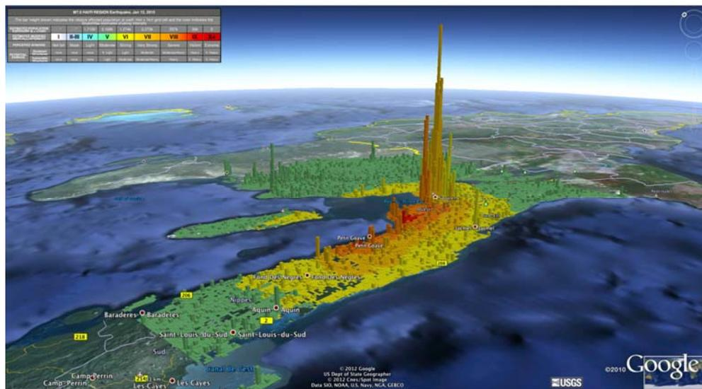
**Figure 2.** PAGER Exposure estimate and its overlay on the LandScan population database in Google Earth for 2010 Haiti earthquake. The bar height indicates the affected population and the color indicates the ShakeMap estimated shaking intensity
