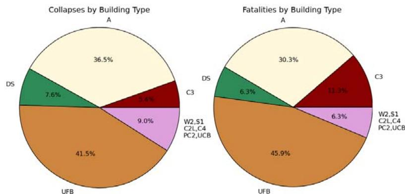
**Figure 4.** Estimated collapse (left) and fatality (right) distribution according to PAGER-STR building typologies (see, Jaiswal and Wald, 2008 for description of PAGER-STR) produced by the semi-empirical model following the M7.1 Van earthquake on October 23, 2011.
