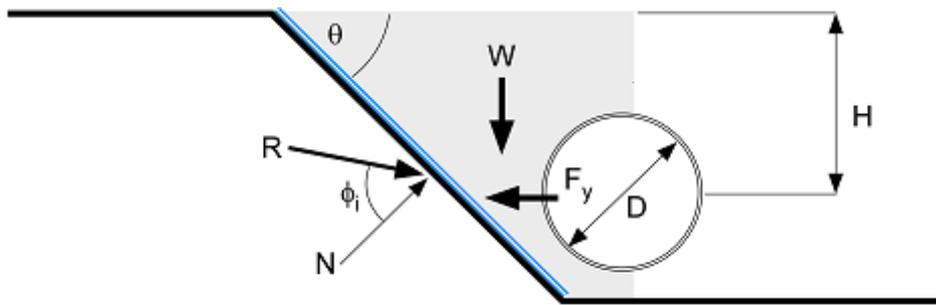
**Figure 5.1** Sliding block mechanism for quantifying  $F_y$  for pipeline systems with geotextile-lined trench walls.  $\phi_i$  is the geotextile-soil interface friction angle.
