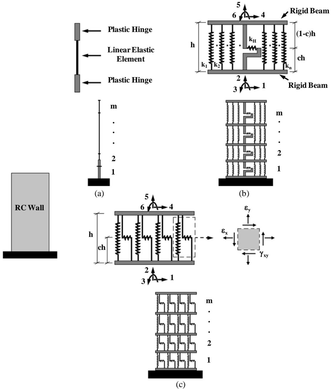
**Figure 2.1.** Macroscopic models and typical shear wall model. ((b) Modified from Orakcal et al. (2004), (c) Modified from Massone et al. (2006))
