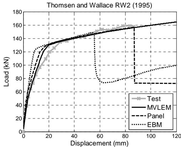
**Figure 4.1.** RW2: Load-displacement response
