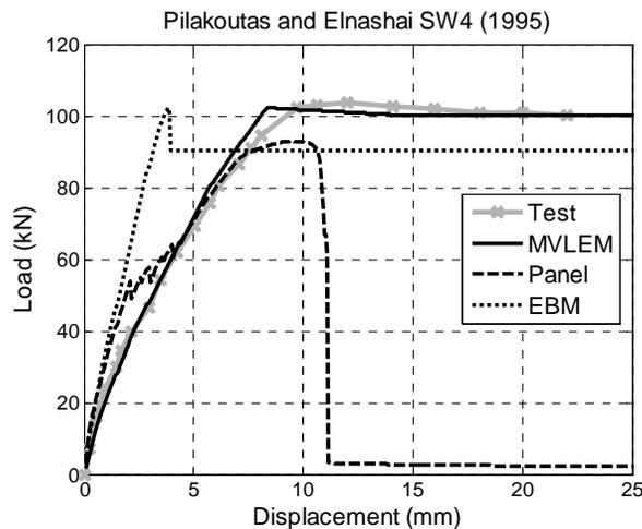
Figure 4.2. SW4: Load-displacement response
