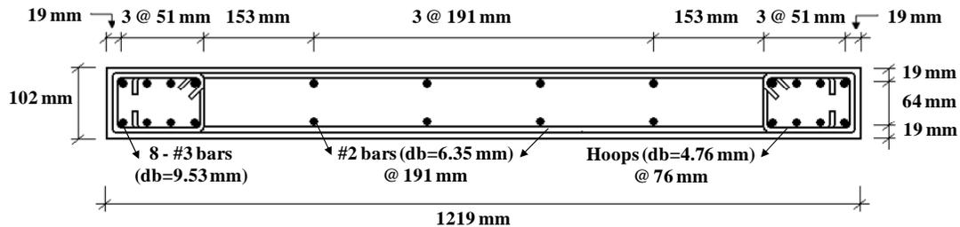
Figure 5.1. Wall cross-section (Modified from Orakcal and Wallace (2004))
