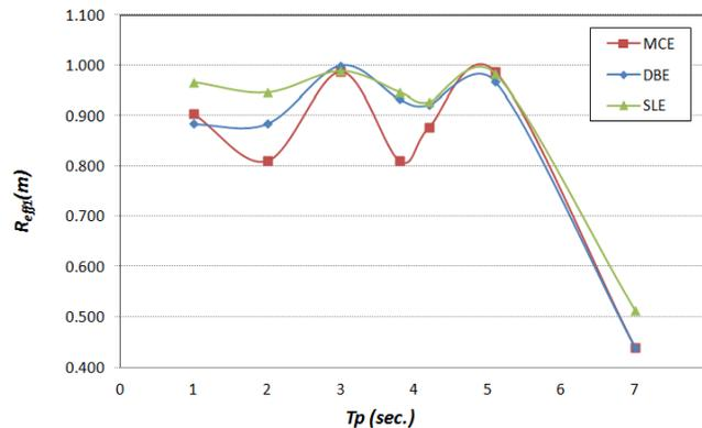
**Figure 6.1.** Optimum values of  $R_{eff1}$  that minimize MRSD in three levels of MCE, DBE and SLE
