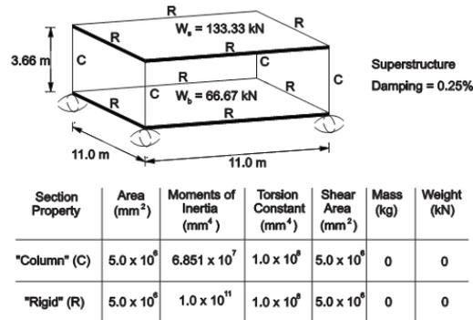
**Figure 3.3.** The isolated superstructure for verification of model (Fenz & Constantinou, 2008)
