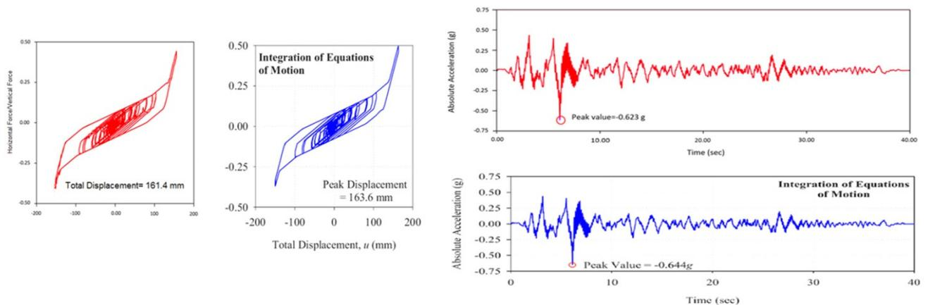
**Figure 3.4.** Comparison of results of TFPB force-displacement and roof acceleration time history from MATLAB analysis (red colours) and results governed by Fenz and Constantinou (Fenz & Constantinou, 2008) (blue colours)
