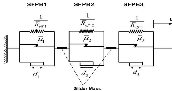
**Figure 3.2.** Three SFPB connected in series to model a TFPB
