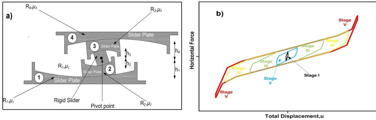
**Figure 3.1.** a) Section of a TFPB, b) Different stages of sliding related to adaptive TFPB
