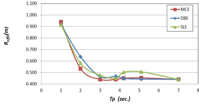
**Figure 6.2.** Optimum values of  $R_{eff1}$  that minimize MDIL in three levels of MCE, DBE and SLE
