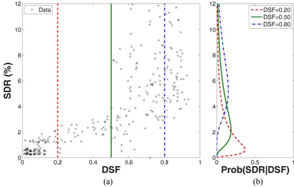
**Figure 3.2.** (a) Scatter plot of DSF versus maximum SDR; (b) Conditional probability density function of SDR given DSF using the two-dimensional kernel for the four-story steel SMRF
