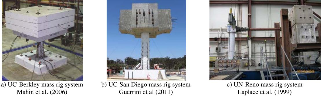
**Figure 1:** Different inertial loading systems used in shake table experiments on RC cantilever columns
