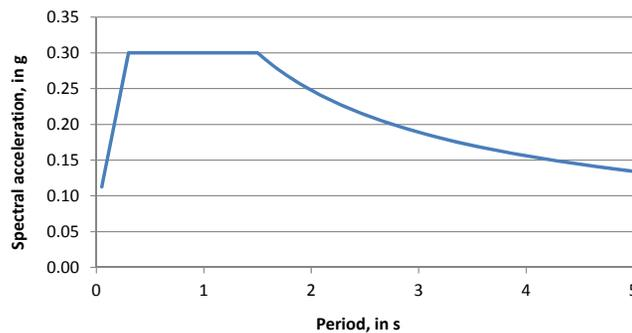
Figure 5. Spectrum regulatory zone B soil type II (CFE, 1993)
