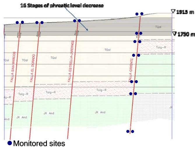
**Figure 7.** Stages of phreatic decrease level process and monitored sites for acceleration spectrums determination
