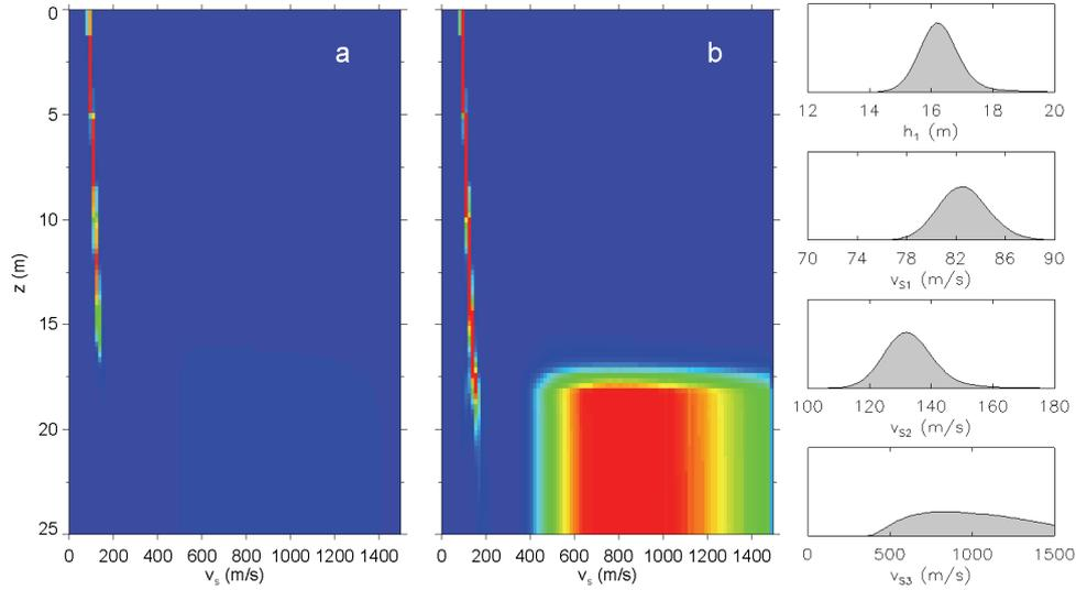
**Figure 3.** Marginal probability  $V_S$  profile for Victoria site fully normalized (left panel) and normalized at each depth (middle panel). The right panel shows 1D marginal distributions of the total thickness of the linear gradient layer ( $h$ ), velocity at the top ( $V_{S1}$ ) and bottom ( $V_{S2}$ ) of the linear layer and in the half-space ( $V_{S3}$ ).
