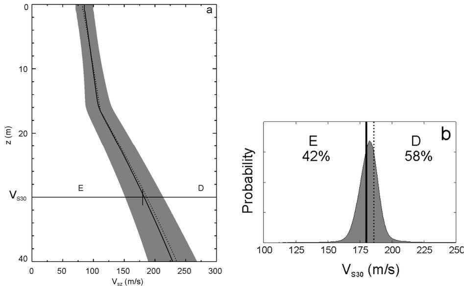
**Figure 6.** (a)  $V_{SZ}$  probability distribution and (b) probability distributions of  $V_{S30}$  for Fraser River delta site 2. MAP model estimate shown by dotted line in both panels Details as in Fig. 4.
