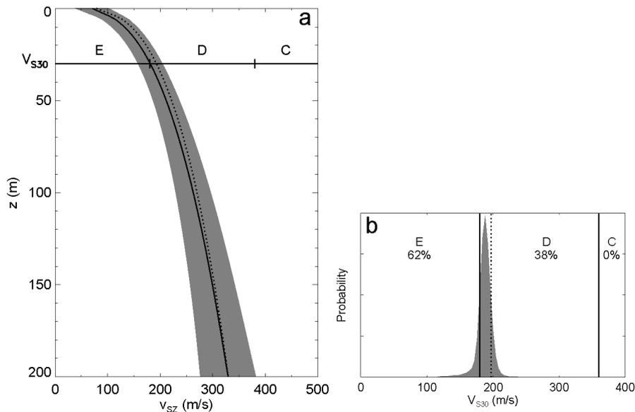
**Figure 5.** (a)  $V_{SZ}$  probability distribution and (b) probability distributions of  $V_{S30}$  for Fraser River delta site 2. MAP model estimate shown by dotted line in both panels. Details as in Fig. 4.
