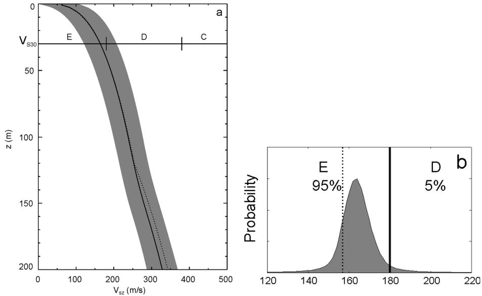
**Figure 4.** (a) Probability distribution for depth-averaged shear-wave velocity  $V_{SZ}$  for Fraser River delta site 1. Solid line represents the mean and shaded region corresponds to mean ± two standard deviations. NEHRP site class boundaries, based on  $V_{S30}$ , are indicated. MAP model  $V_{SZ}$  profile shown by dotted line. (b) Probability distributions of  $V_{S30}$ . MAP model  $V_{S30}$  estimate shown by dotted line.
