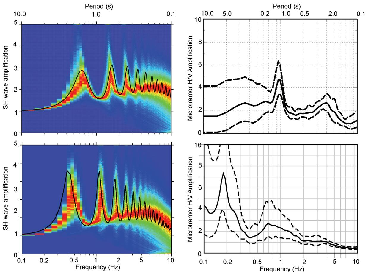
**Figure 7.** Left panels: Marginal probability amplification spectra for delta site 1 (top) and 2 (bottom) calculated from the sample of  $V_S$  profiles shown in Fig. 1 and 2, respectively. Black line corresponds to spectrum predicted for the most-probable  $V_S$  profile. Right panels: Average microtremor H/V spectral ratio (dashed lines denote  $\pm$  two standard deviations) for delta site 1 (top) and 2 (bottom).
