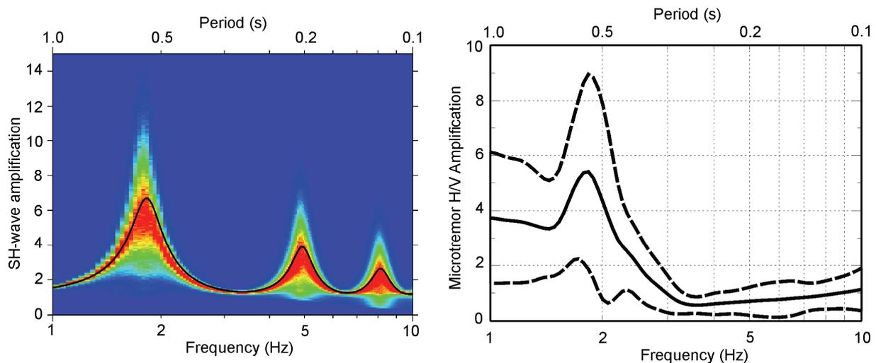
**Figure 9.** Left panel: SH-wave amplification probability distributions for the Victoria site calculated for the  $V_S$  probability distribution shown in Fig. 3. Right panel: Average microtremor H/V spectral ratio (dashed line) and  $\pm$  two standard deviations (solid lines).
