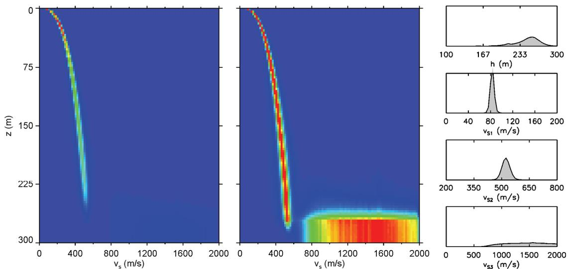
**Figure 2.** Marginal probability  $V_S$  profile for Fraser River delta site 2 fully normalized (left panel) and normalized at each depth (middle panel). The right panel shows 1D marginal distributions of the total thickness of the powerlaw layer ( $h$ ), velocity at the top ( $V_{S1}$ ) and bottom ( $V_{S2}$ ) of the powerlaw gradient layer and in the
