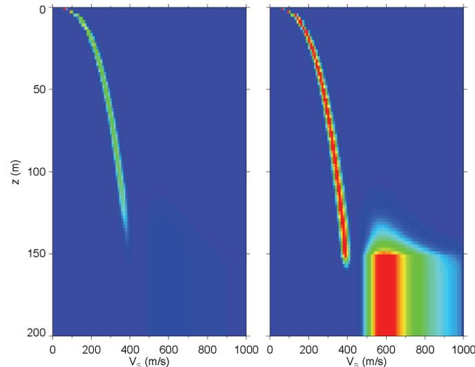
**Figure 1.** Marginal probability  $V_S$  profile for Fraser River delta site 1 fully normalized (left panel) and normalized at each depth (right panel).
