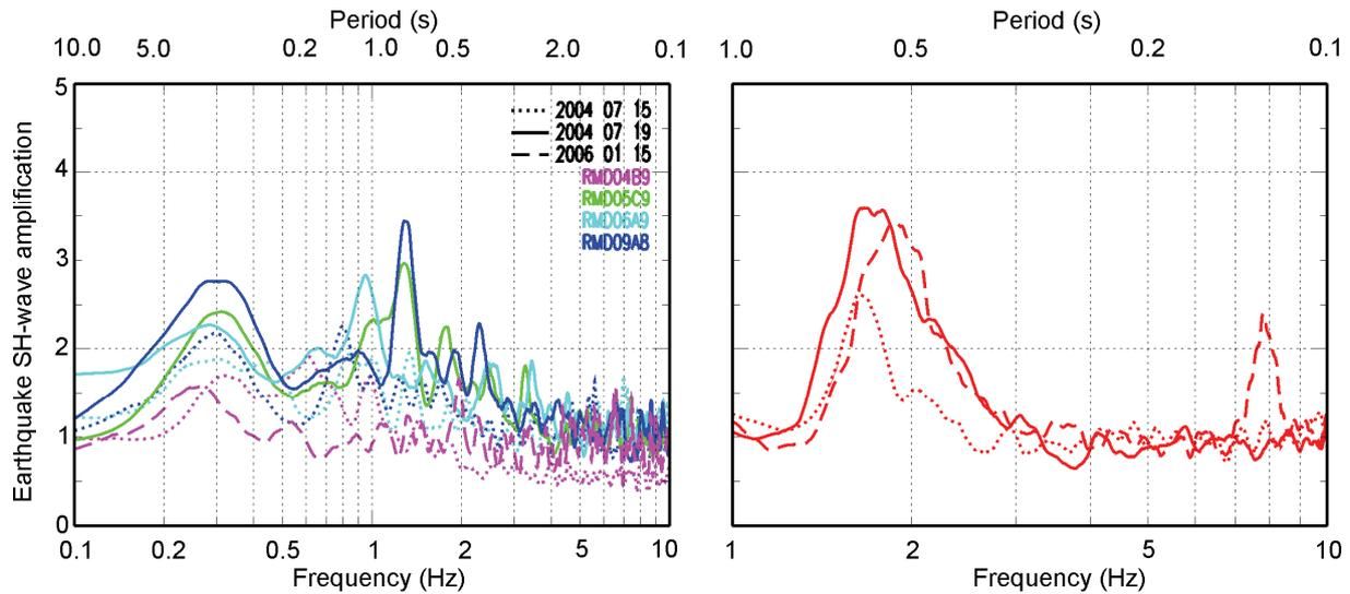
**Figure 8.** Earthquake SH/V ratios from three events recorded at four Geological Survey of Canada strong-motion stations on the delta (left panel; station names given in legend) and at the Victoria site (right panel).
