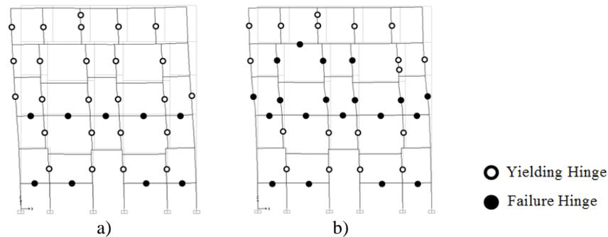
**Figure 10.** Structure deformed shape: a) Step 15 ( $d_{t,65\%}=0.028m$ ); b) Step 34 ( $d_t=0.047m$ ).
