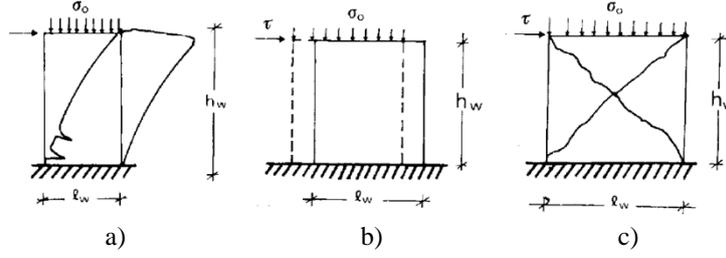
**Figure 3.** Failure mechanisms of a masonry pier (Pasticier *et al.*, 2008): a) rocking, b) sliding shear, c) diagonal shear cracking.
