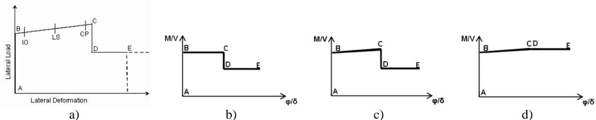
**Figure 5.** Plastic Hinge (Demirél, 2010): a) SAP2000 hinge definition; b) hinge with perfectly plastic behaviour – Case 1; c) hinge with post elastic stiffness – Case 2; d) hinge with post elastic stiffness without final strength loss – Case 3.
