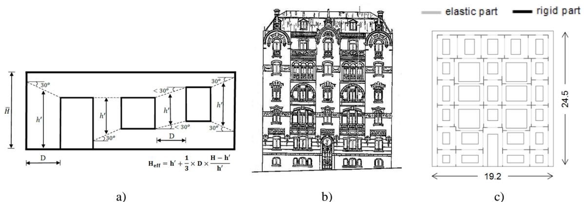
**Figure 2.** a) Effective height determination proposed by Dolce (Dolce, 1989); b) Façade wall of the building and c) Equivalent Frame Model (dimensions in m).
