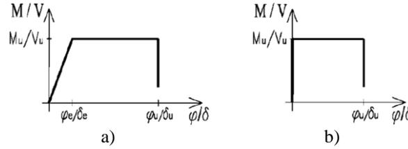
**Figure 4.** Masonry Piers (Pasticier *et al.*, 2008): a) Elasto-plastic behaviour of the element, b) Plastic hinge behaviour.
