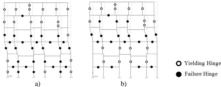
**Figure 7.** Plastic hinges distribution at the final stage of Case 3: a) Uniform Load; b) Modal Load.
