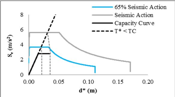
**Figure 8.** Acceleration-Displacement Response Spectra (Short Period Range).
