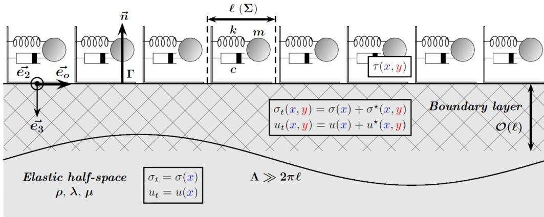
**Figure 2.1** Elastic half-space loaded by periodic distribution of horizontal one-degree-of-freedom-oscillators
