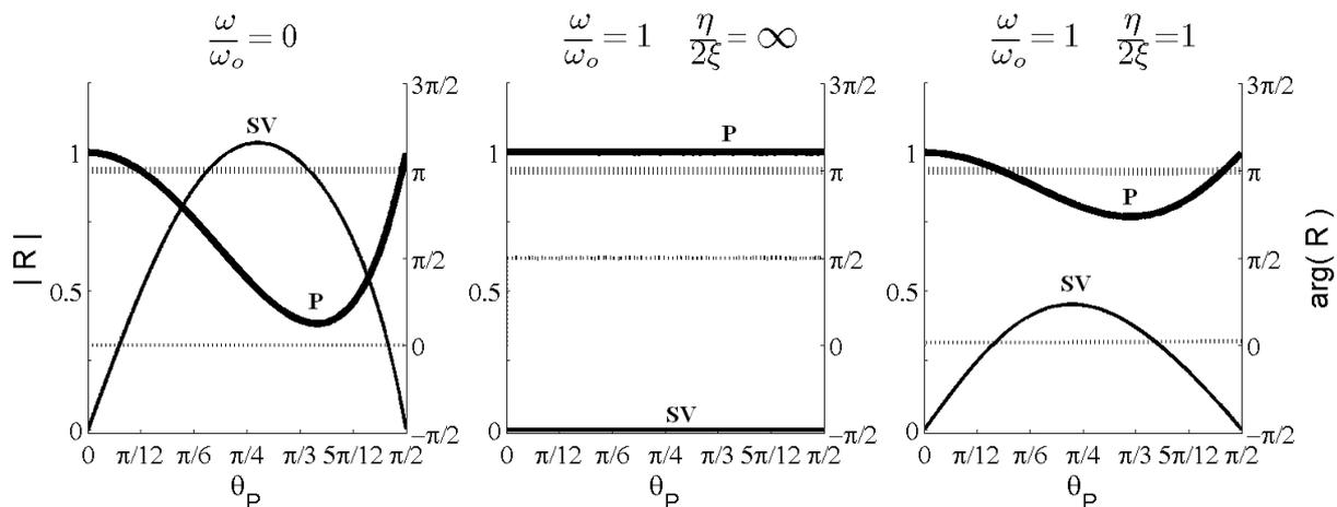
**Figure 3.5** Modulus of the coefficient of reflection in the case of an incident P wave which incident plane contains the resonant direction  $e_o$ . Calculations performed with  $\nu = 1/3$ ,  $\eta = 10\%$  and  $2\xi = 0\%$  or  $10\%$
