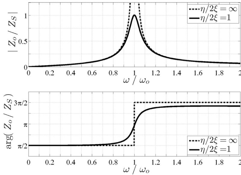
**Figure 2.2** Ratio between the surface impedance  $Z_0$  in the resonant direction and the impedance  $Z_S$  of the medium for shear waves. Calculations performed with  $\eta=10\%$  and  $2\xi=0\%$  or  $10\%$
