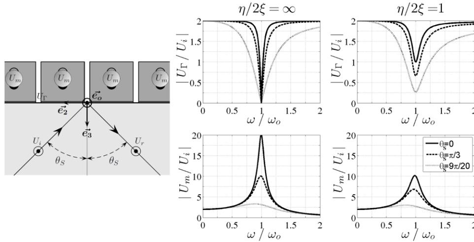
**Figure 3.1** Surface displacement (top) and oscillators' displacement (bottom) in the resonant direction for a unitary incident SH wave polarized along the resonant direction. Calculations performed with  $\eta = 10\%$  and  $2\xi = 0\%$  or  $10\%$
