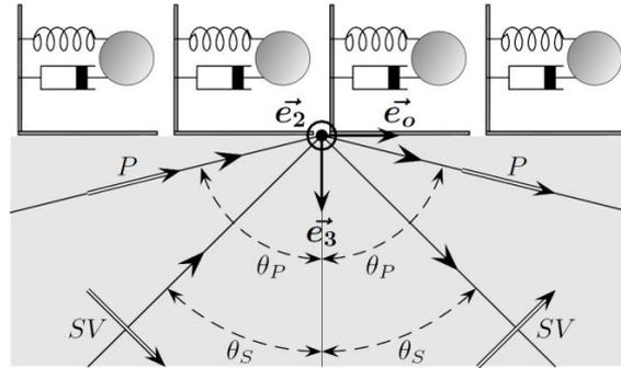
**Figure 3.4** Reflection of SV and P waves which incident plane contains the resonant direction  $e_o$ .
