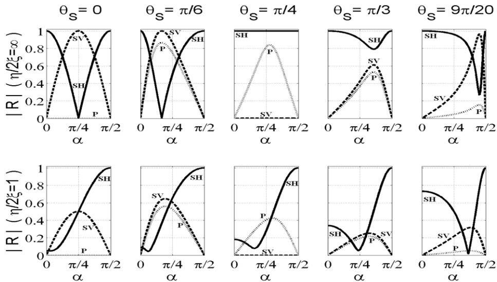
**Figure 4.4** Modulus of the coefficients of reflection at the resonance of the oscillators for a  $\theta_s$ -incident SH wave which polarization makes an angle  $\alpha$  with the resonant direction  $e_o$ . Calculations performed with  $\nu=1/3$ ,  $\eta=10\%$  and  $2\xi=0\%$  or  $10\%$
