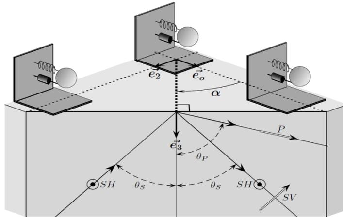
**Figure 4.3** SH wave which polarisation makes an angle  $\alpha$  with the resonant direction  $e_o$  and incoming with an incidence  $\theta_s$
