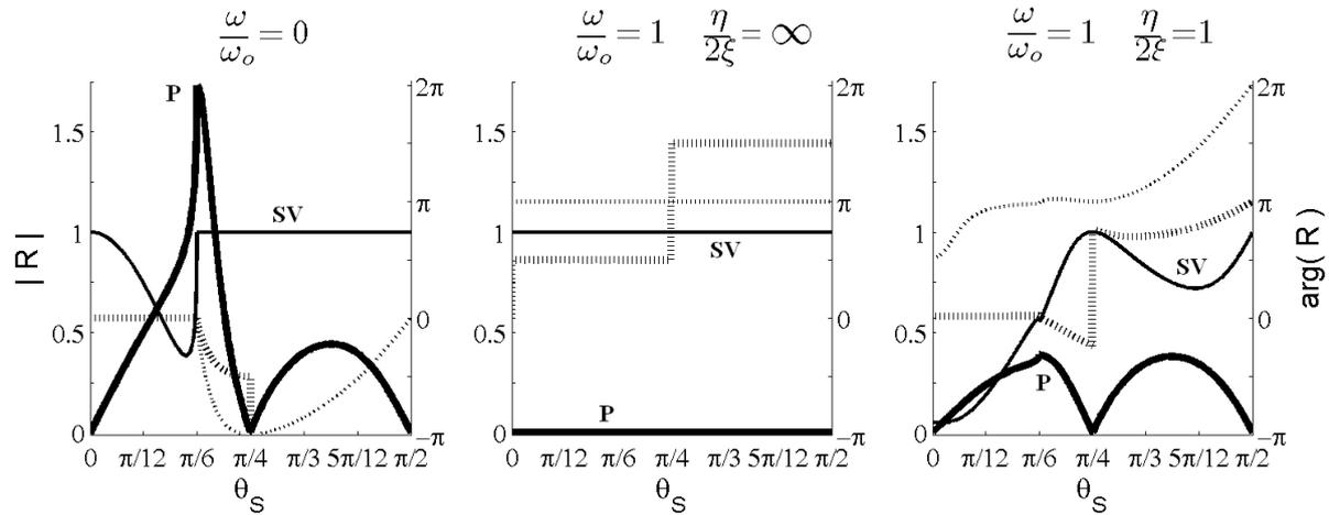
**Figure 3.6** Modulus of the coefficient of reflection in the case of an incident SV wave which incident plane contains the resonant direction  $e_o$ . Calculations performed with  $\nu = 1/3$ ,  $\eta = 10\%$  and  $2\xi = 0\%$  or  $10\%$
