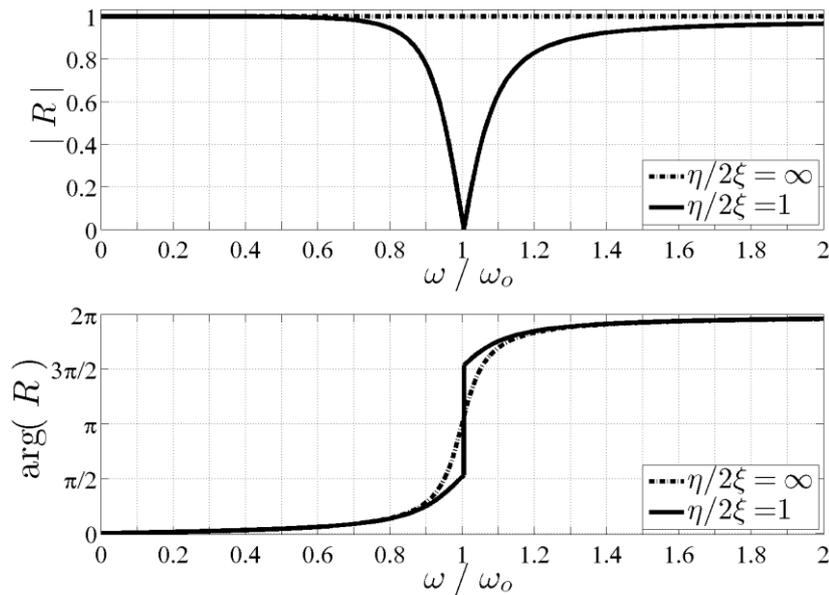
**Figure 4.2** Coefficient of reflection  $R$  of a normally-incident shear wave polarized in the resonant direction. Calculations performed with  $\eta=10\%$  and  $2\xi=0\%$  or  $10\%$
