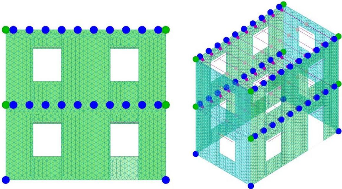
**Figure 6.** Front view and 3d view of the model with Acca Edilus
