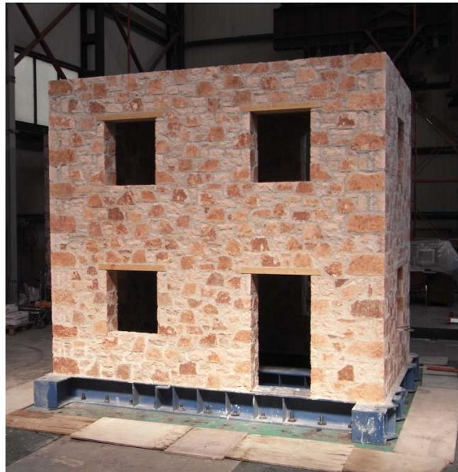
**Figure 1.** Floor plan and photo of the specimen on shaking table
