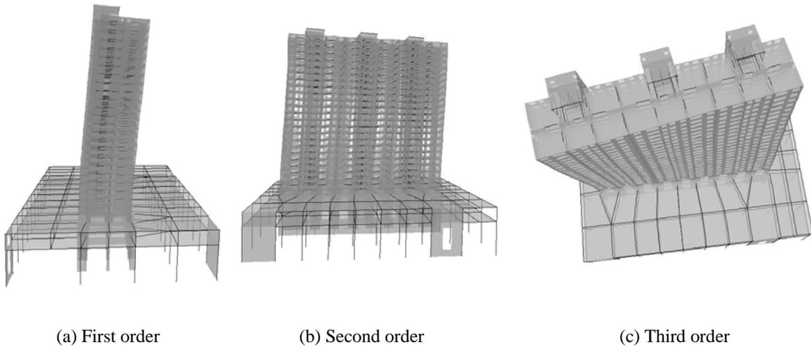
**Figure 4.2.** First three vibration modes
