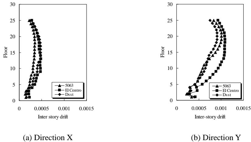
**Figure 4.4.** Analytical results of inter-story drift
