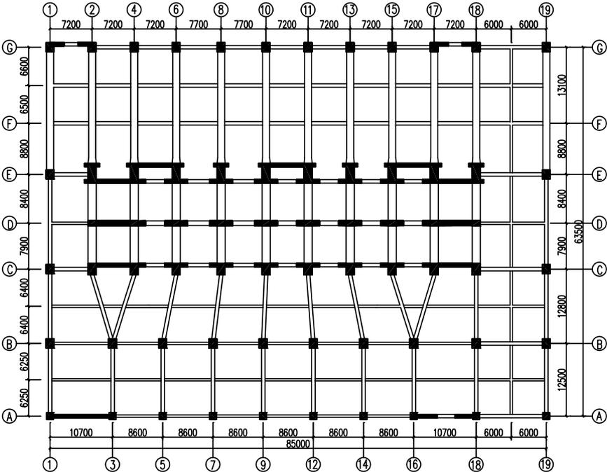
Figure 2.1. Structural plan of the first floor
