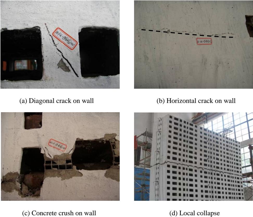
**Figure 4.1.** Typical failure pattern
