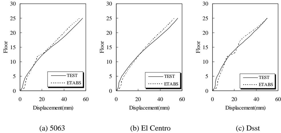
**Figure 4.3.** Envelopes of story displacement response in Y direction
