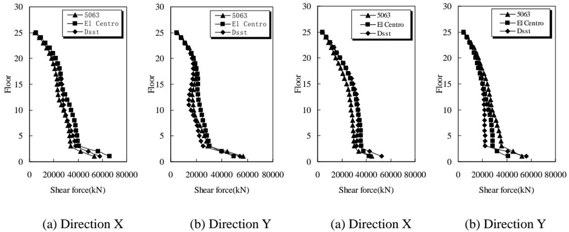
**Figure 4.5.** Analytical results of story shear distribution    **Figure 4.6.** Test results of story shear distribution
