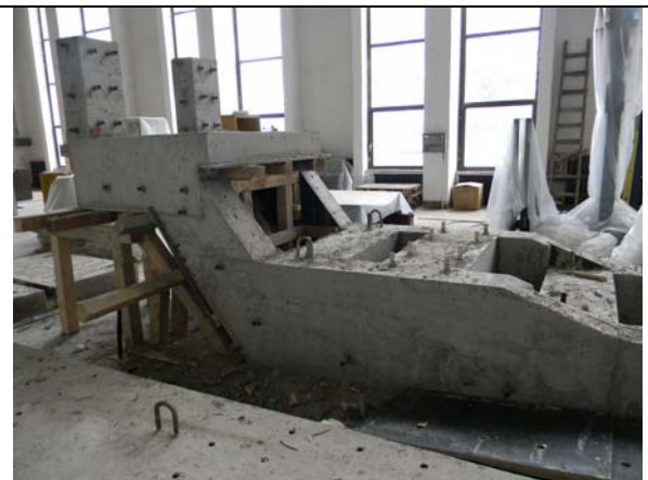
Figure 10. Erected large-scale experimental bridge model in IZIIS, Skopje, laboratory (phase-1)
