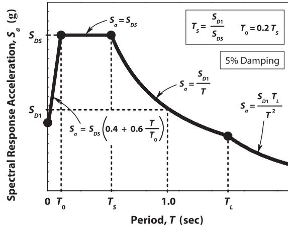
**Figure 1-2.** 2012 IBC and ASCE 7-10 design earthquake response spectrum that define the seismic ground motion demand requirements for building structures
