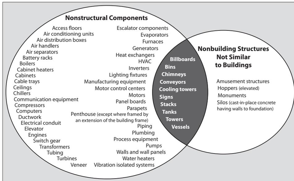
Figure 1-1. Overlap of nonstructural components and nonbuilding structures
