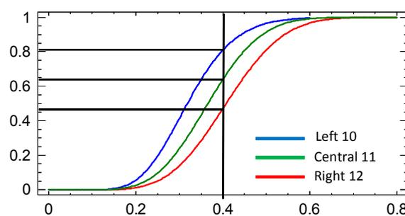
**Figure 8.** Fragility curves of piers of Motín de Oro Bridge. Seismic scenario 1
