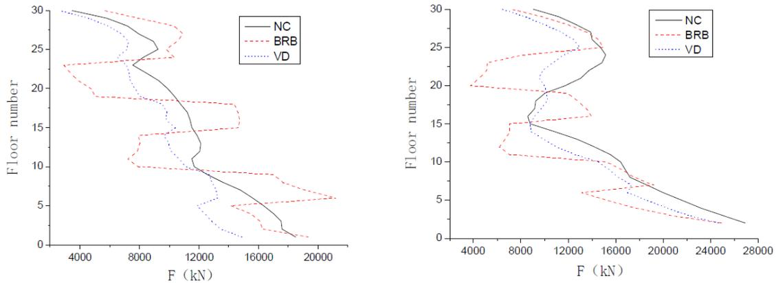
**Fig. 4.** Story shear force of structures
