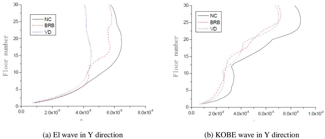
**Fig. 3.** Inter-story displacement angle of structures
