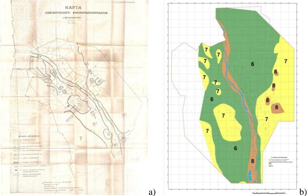
Figure 1. The map of seismic microzonation of 1970: original (a), GIS-project (b)
