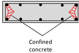
**Figure 9.** Confined concrete are at the stirrups level in the 55x15 shear wall
