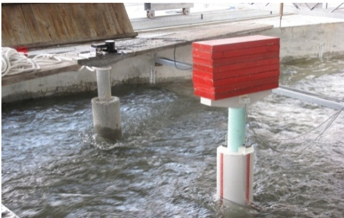
Figure 1. Single bridge column experiment
