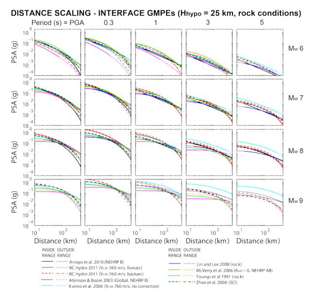
**Figure 3.** Trellis chart showing decay of predicted PSAs for pre-selected subduction GMPEs for various structural periods and magnitudes for rock site conditions. Dashed lines indicated where the scenario falls outside the magnitude-distance range of validity of the model.
