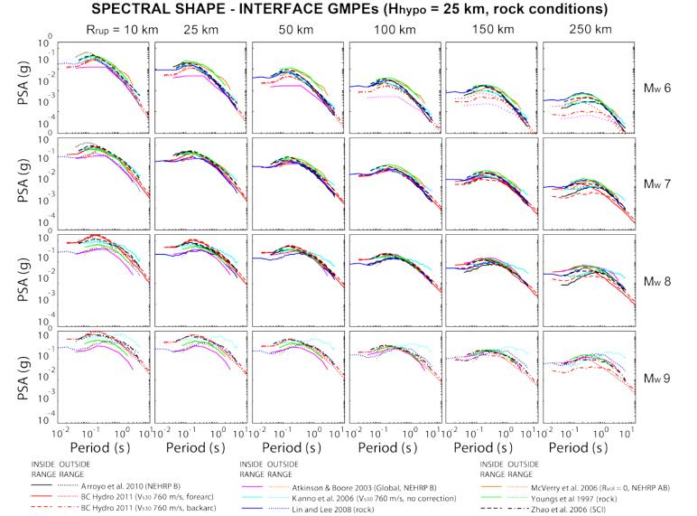
Figure 1. Trellis chart showing predicted PSAs for pre-selected subduction GMPEs for various interface earthquake scenarios for rock site conditions. Dashed lines indicated where the scenario falls outside the magnitude-distance range of validity of the model.
