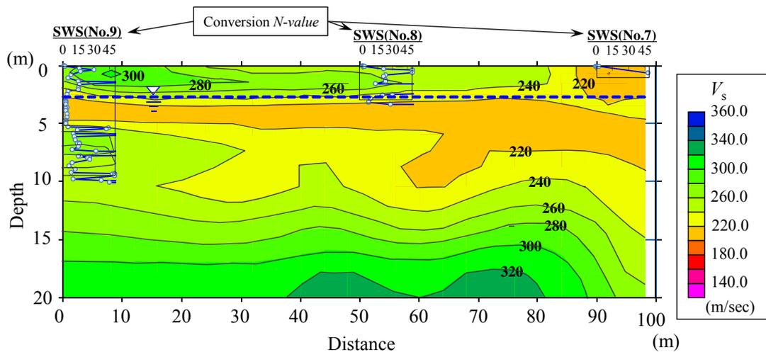
**Figure 5.** Surface wave exploration result (SWE-3w survey line)
