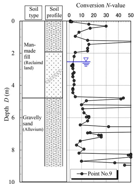
Figure 4. Soil profile at Hirogawa Island (Point No.9)
