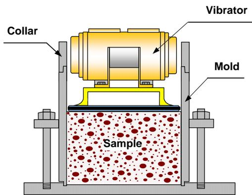
**Figure 8.** Minimum and Maximum density test apparatus
