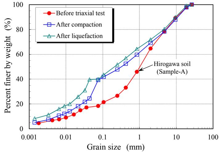
**Figure 16.** Comparison of grain size distribution curve
