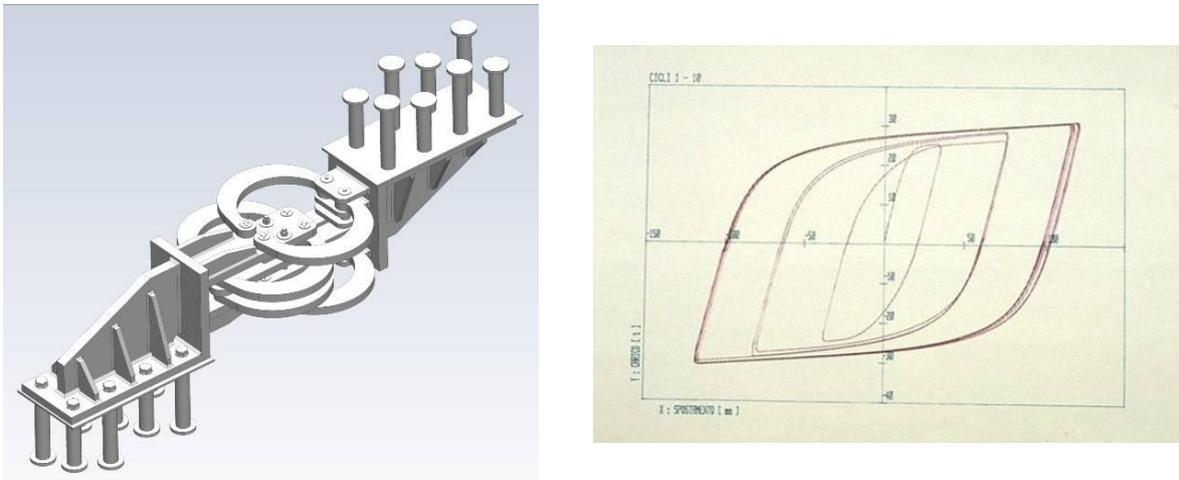
**Figure 6.** Hysteretic device installed on the ramps abutments and typical force-displacement loop
