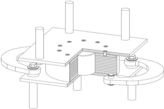
**Figure 10.** LRB coupled with transversal hysteretic C-shaped elements for the ramps of PS3-PS4
