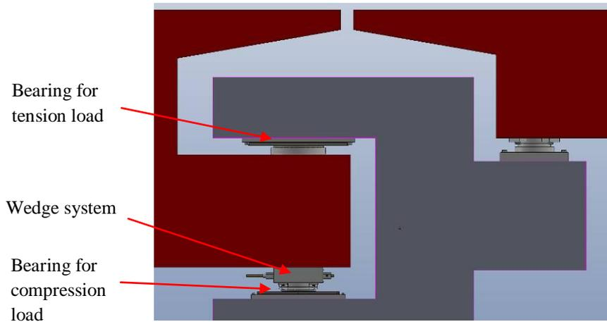
**Figure 4.** Spherical bearings coupled to carry both compressive and tensile vertical load
