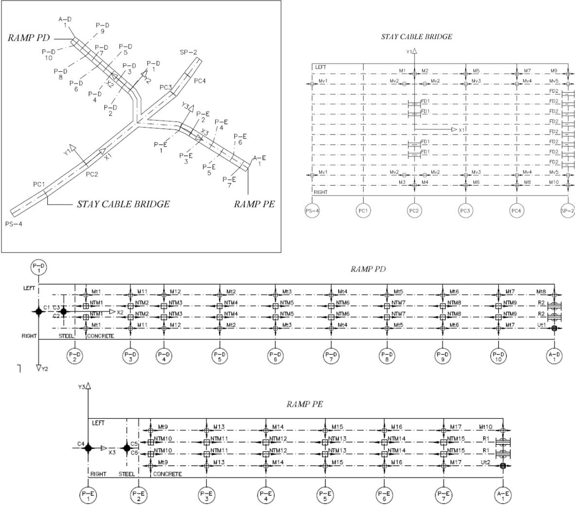
Figure 3. Bearing layout stay cable bridge
