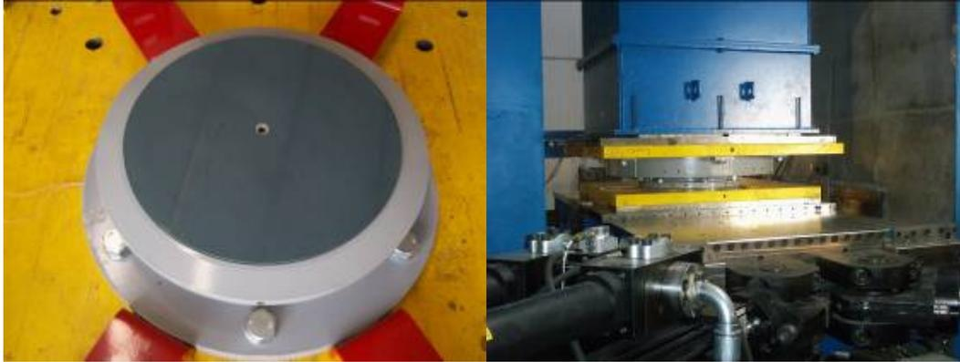
**Figure 6.** Friction pendulum with its high friction sliding material and tests performed
