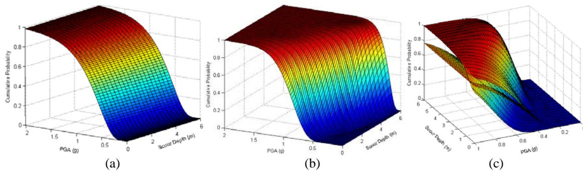
**Figure 3.4** Combined fragility surface of continuous concrete box-girder bridge under earthquake and scour
