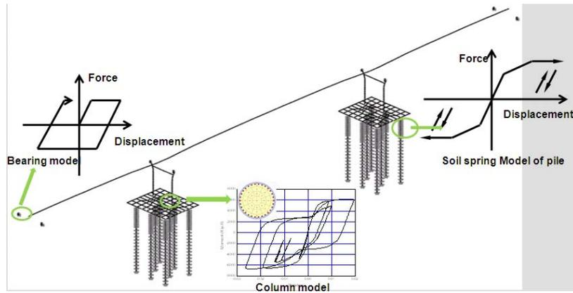
**Figure 3.3** The analytical model
