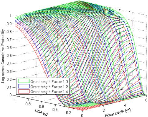
**Figure 3.5** Combined fragility surface for different overstrength factors under earthquake and scour hazards
