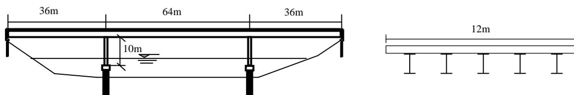
**Figure 3.2** Schematic of three span continuous steel-girder with concrete-deck bridge
