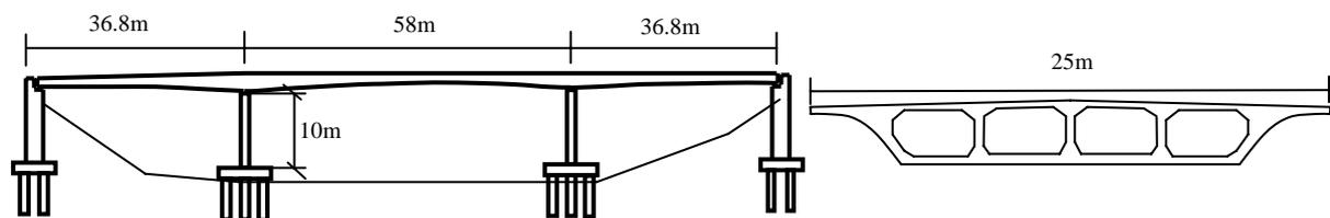
**Figure 3.1** Schematic of three span continuous concrete box-girder bridge
