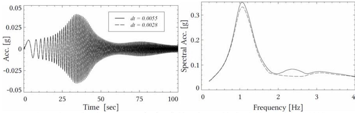
**Figure 6.** Acceleration responses for free field analyses with  $dt = 0.0055$  and  $dt = 0.0028\text{ s}$
