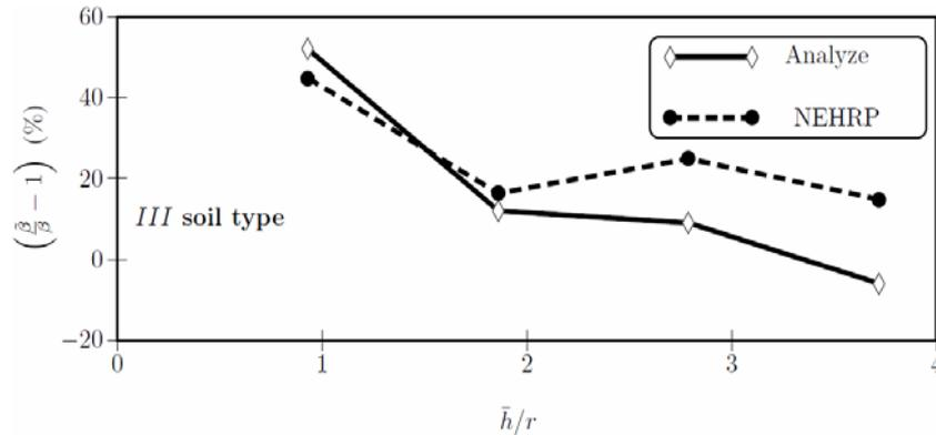
**Figure 11.** Variations of structural damping with  $\bar{h}/r$  (soil type III)
