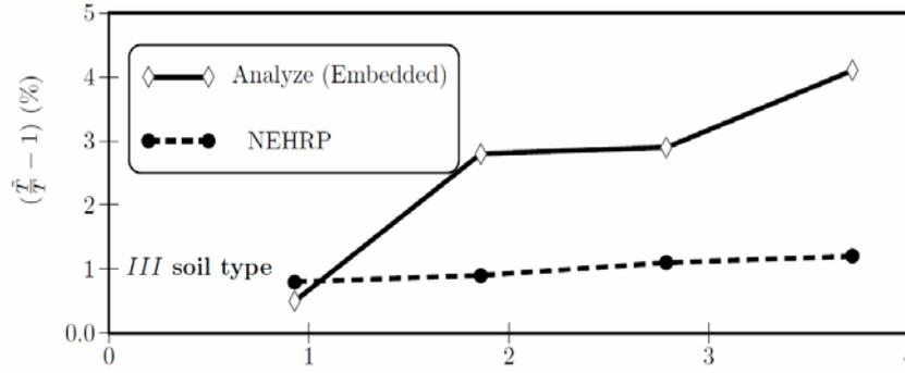
**Figure 10.** Variation of fundamental periods with  $\bar{h}/r$  ratios in embedded foundations
