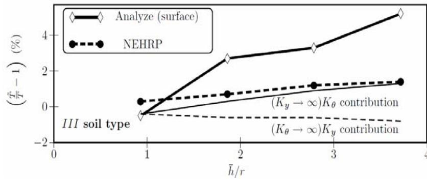
**Figure 8.** Variation of fundamental periods with  $\bar{h}/r$  ratios in surface foundations (soil type III)
