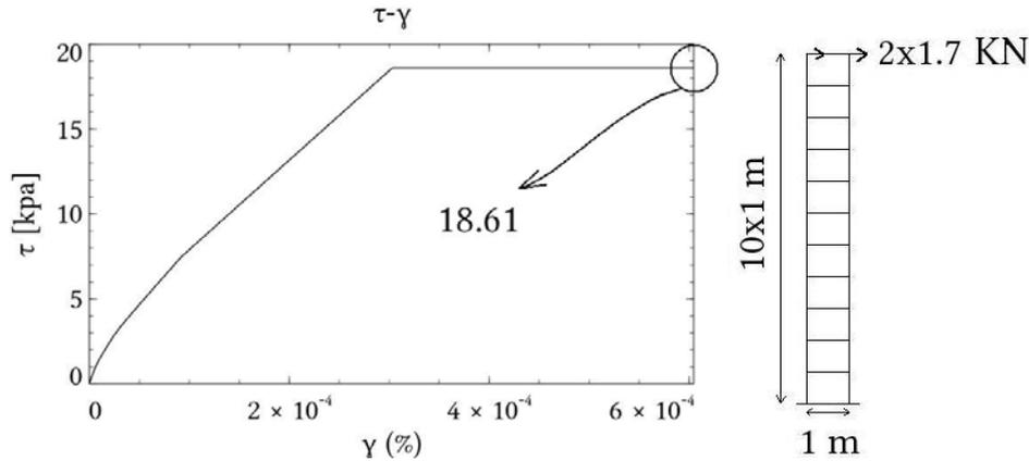
**Figure 4.** Shear stress-strain obtained from pushover analyses
