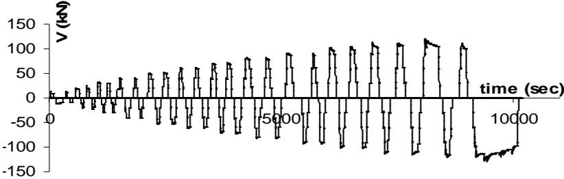
Figure 1.2. Time history of the horizontal force for the specimen B3
