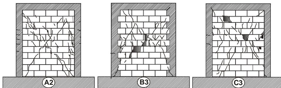
Figure 2.1 Final crack patterns
