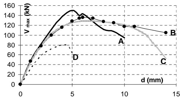
Figure 2.4 Average measured resistant force for series A, B and C
