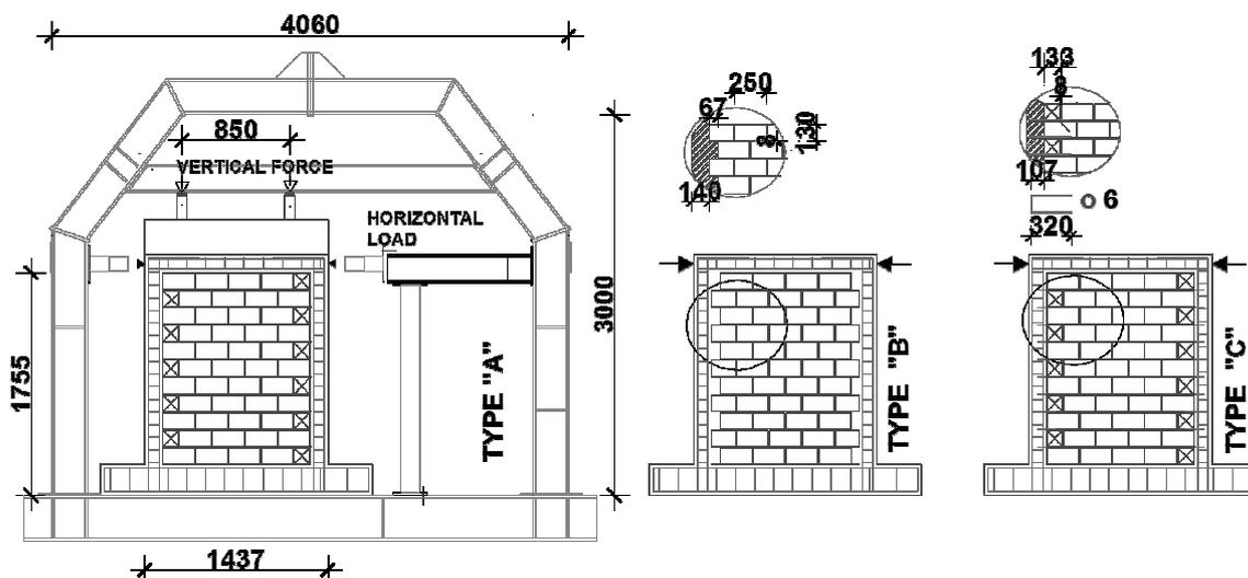
**Figure 1.1.** Test equipment and three different types of specimens
