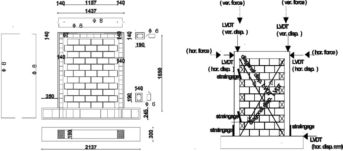
Figure 1.3 Outline of test specimen and measured values
