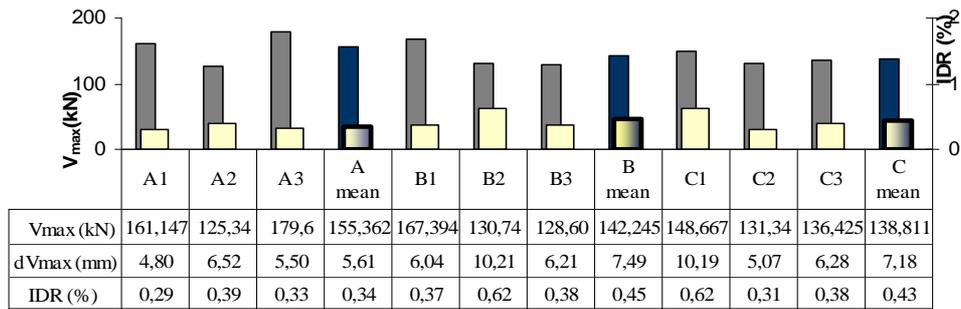
Figure 2.3 Comparison of the maximum horizontal resistance force, models A1-C3
