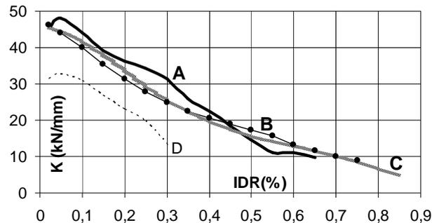
Figure 2.5 Deterioration of secant stiffness for series A,B and C
