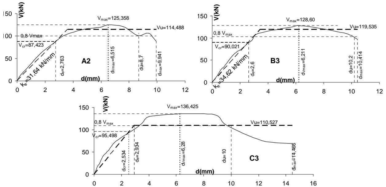
Figure 2.5 Experimentally obtained and idealized hysteresis envelopes for one specimen of series A,B and C
