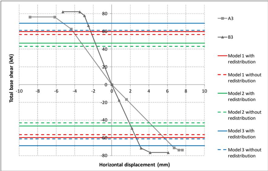
Figure 5.2 Comparison of theoretical models with test results
