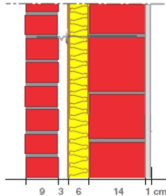
**Figure 1.1.** Typical structure of Belgian masonry walls.
