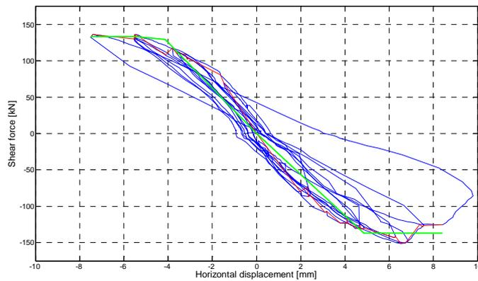
**Figure 4.1.** Horizontal cyclic behaviour of the full wall.
