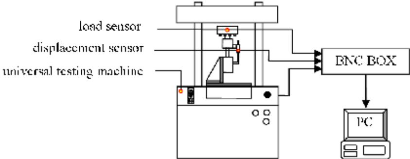
Figure 4. Layout of Experiment of Shockproof Fixed Feet
