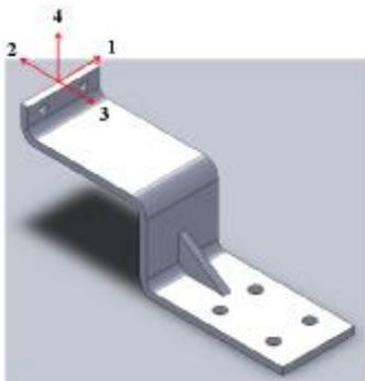
Figure 5. Define Z-type with Directions of the Experiment
