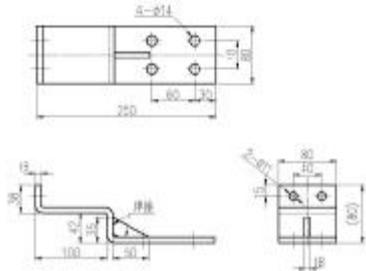
Figure2. Z-type of shockproof fixed foot
