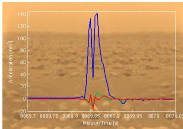
**Figure 2.** Data of “Huygens Spacecraft” accelerometer while landing on Titan's surface
