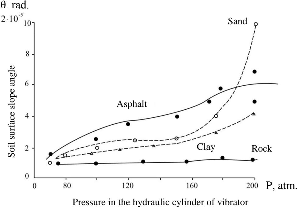
Figure 7. The effect of pressure in the hydraulic cylinder of the vibrator on seismic radiating effect of soil slope from the distance to the source (P. Uznosh, Belarus, 1992; city Dedoplistskaro, Georgia, 1992)
