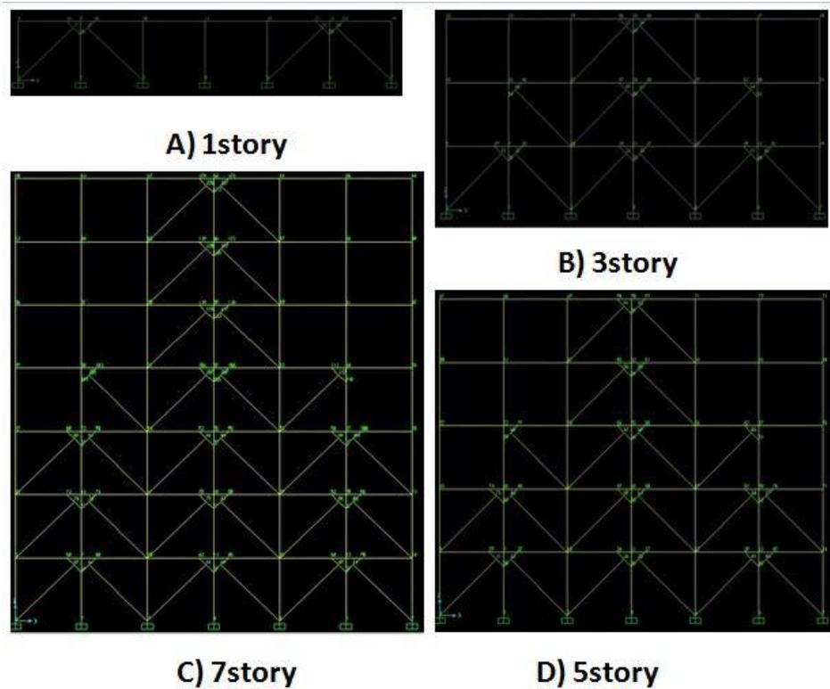
**Figure 2.6.** Layout of (A) 1story (B) 3story (C) 7story (D) 5story braced frames
