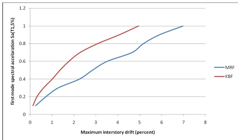
**Figure 4.4.** IDA curves for 5story Moment Resisting Frame and Knee Braced Frame
