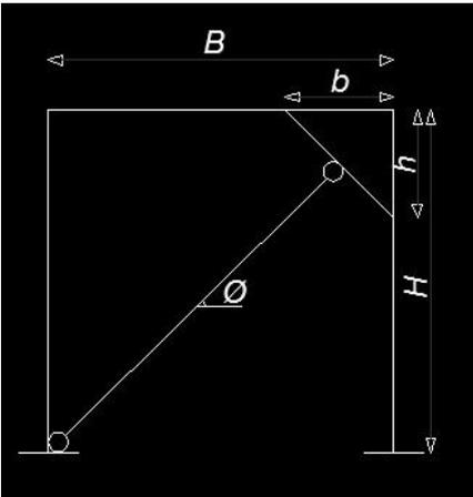
Figure 2.4. One story frame retrofitted by knee brace
