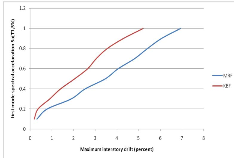
**Figure 4.5.** IDA curves for 7story Moment Resisting Frame and Knee Braced Frame
