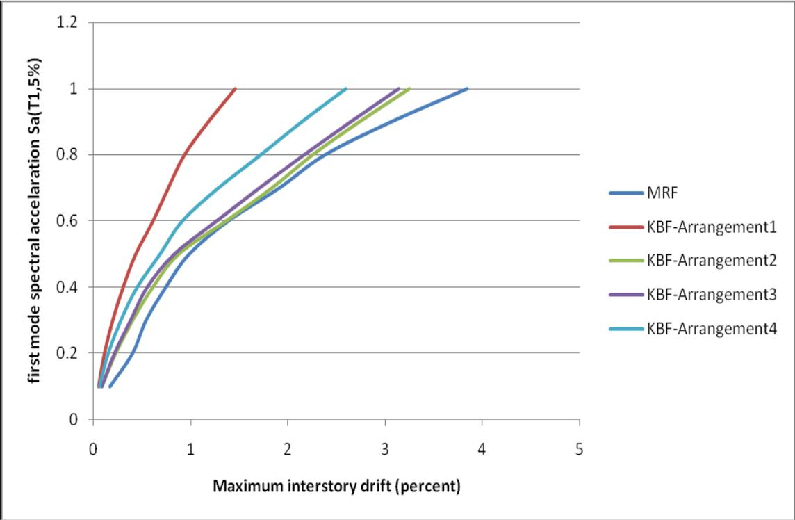
Figure 4.1. IDA curves for 3story buildings with different arrangement of braces
