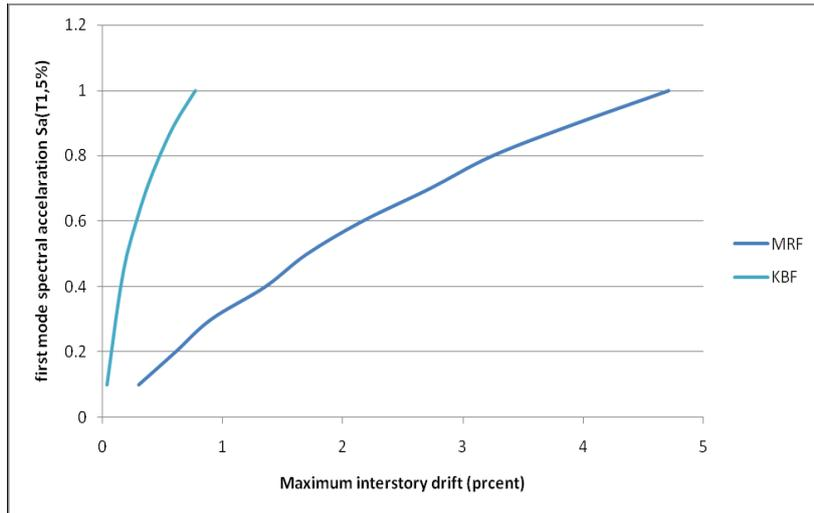
**Figure 4.2.** IDA curves for 1story Moment Resisting Frame and Knee Braced Frame
