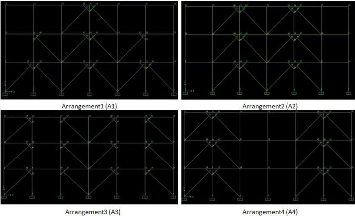
Figure 2.5. Layout of braced frames with different distribution of braces
