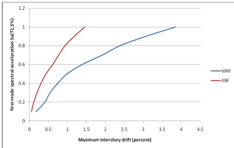
**Figure 4.3.** IDA curves for 3story Moment Resisting Frame and Knee Braced Frame
