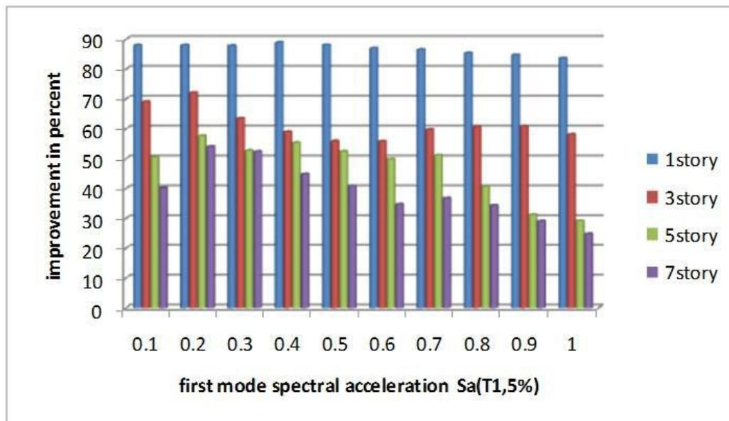
**Figure 4.6.** Reduction of drift due to using knee braces
