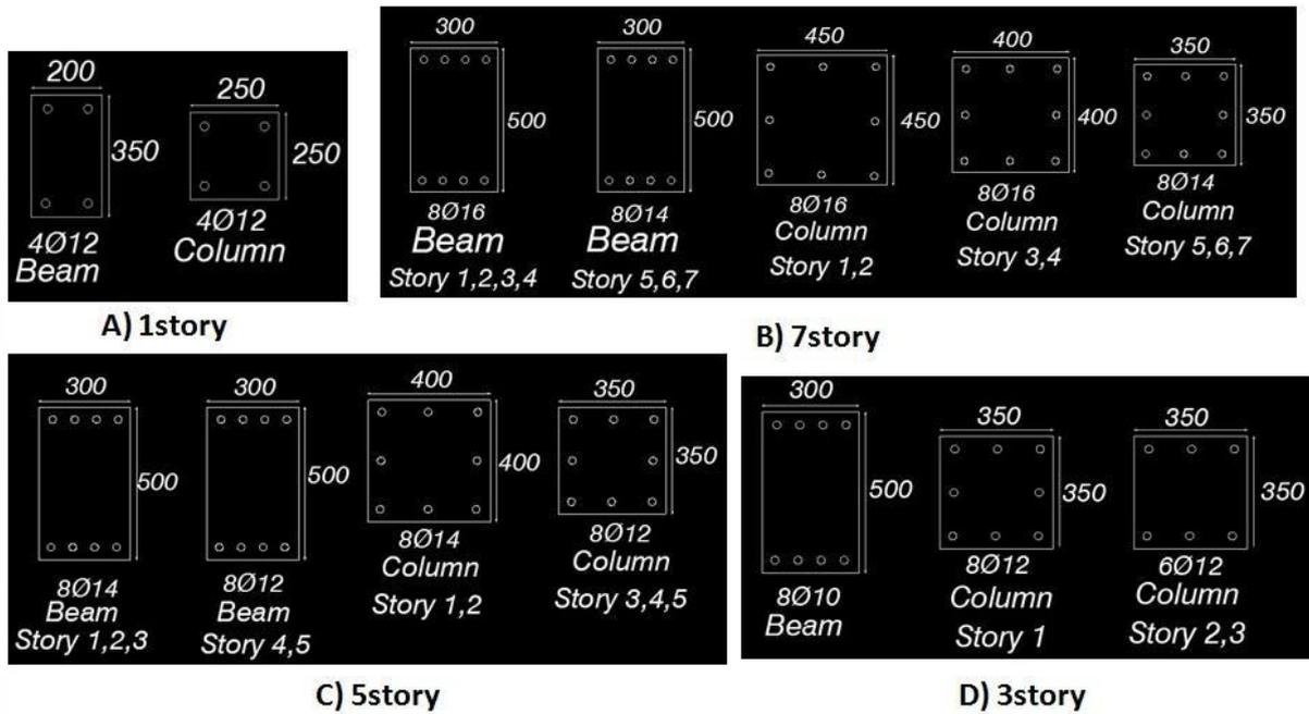
Figure 2.3. Section of beams and columns (in mm) in (A) 1story (B) 7story (C) 5story (D) 3story buildings
