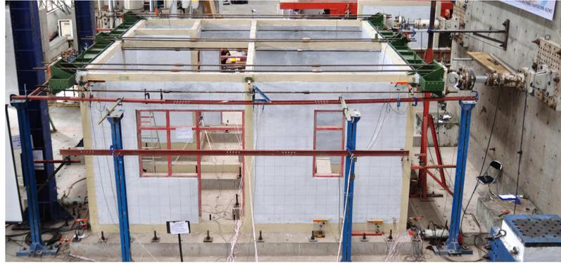
**Figure 3.1.** Plan view and photo of the masonry house model
