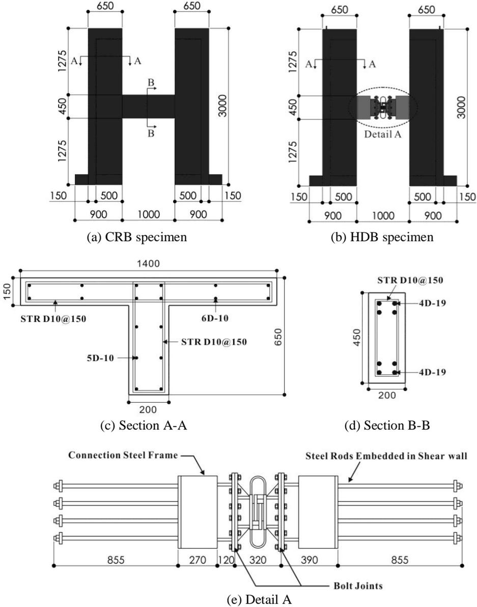
Figure 3.1 Dimensions and connection details of test specimens
