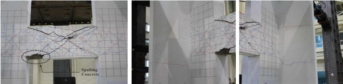
(c) Crack patterns for CRB specimen
