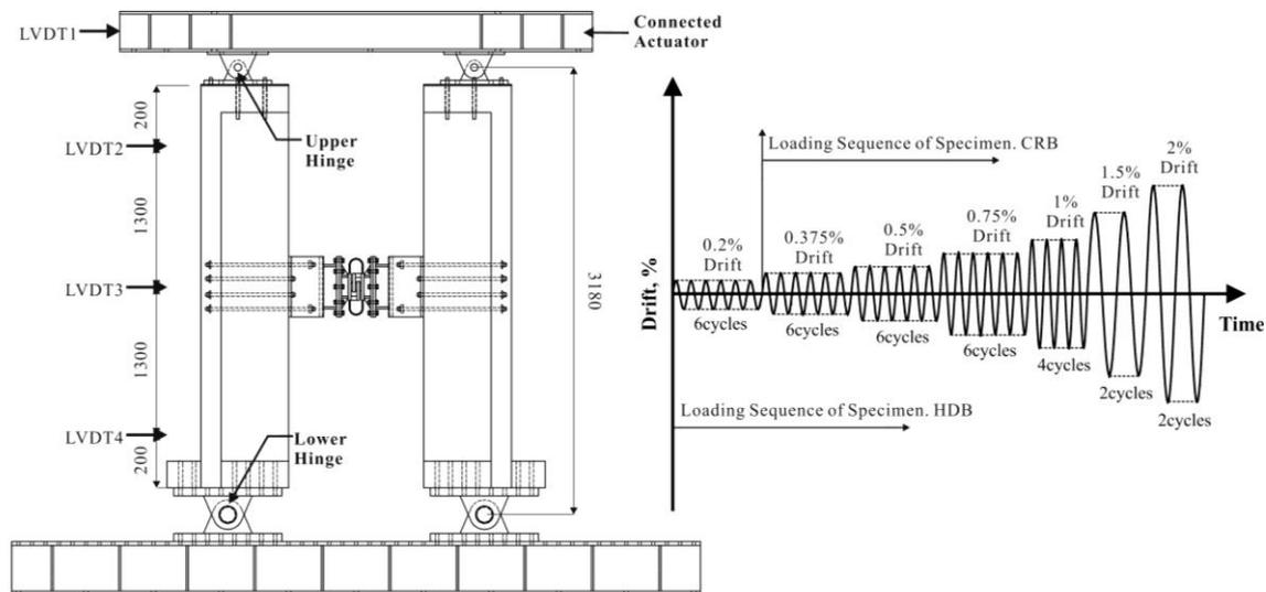
**Figure 3.2** Testing setup, instrumentation and loading sequence
