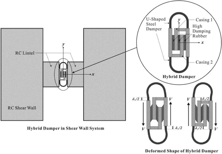
**Figure 2.1** Schematic drawing of a hybrid damper embedded into a coupling beam connecting RC shear walls and the deformed shapes of a hybrid damper
