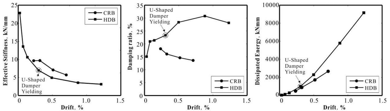
**Figure 3.4** Comparison of seismic performance indexes
