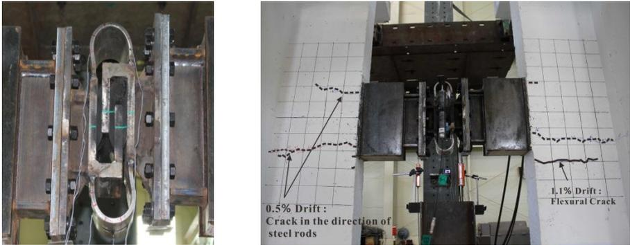
(d) Deformed shape of hybrid damper and crack patterns for HDB specimen
