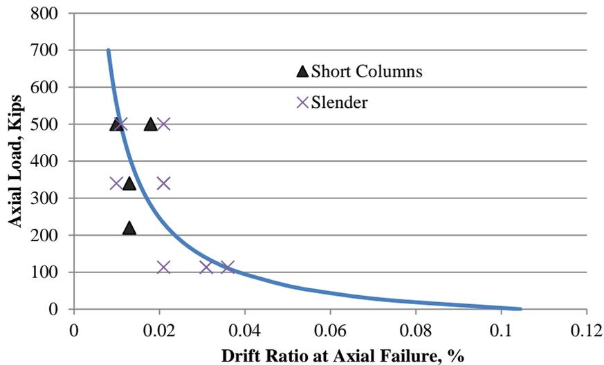
**Figure 4.** Comparison between measured and calculated drift ratio at axial failure for column specimens tested at UC-Berkeley and as part of the PEER-NSF project.
