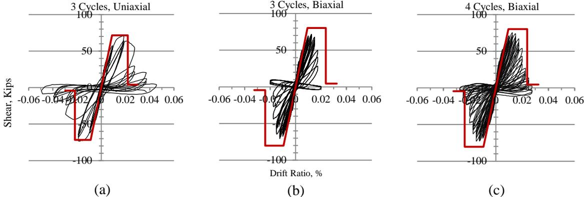
**Figure 6.** Hysteretic response of three columns subjected to different displacement histories. All columns had a longitudinal reinforcement ratio of 2.5%, diamond and rectangular ties spaced at 12 in., and an axial load of 150 Kips.
