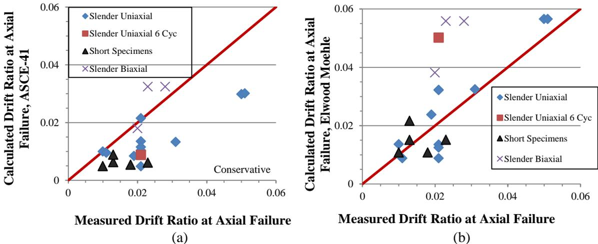
**Figure 3.** Comparison between measured and calculated drift ratio at axial failure for column specimens tested at UC-Berkeley and as part of the PEER-NSF project.
