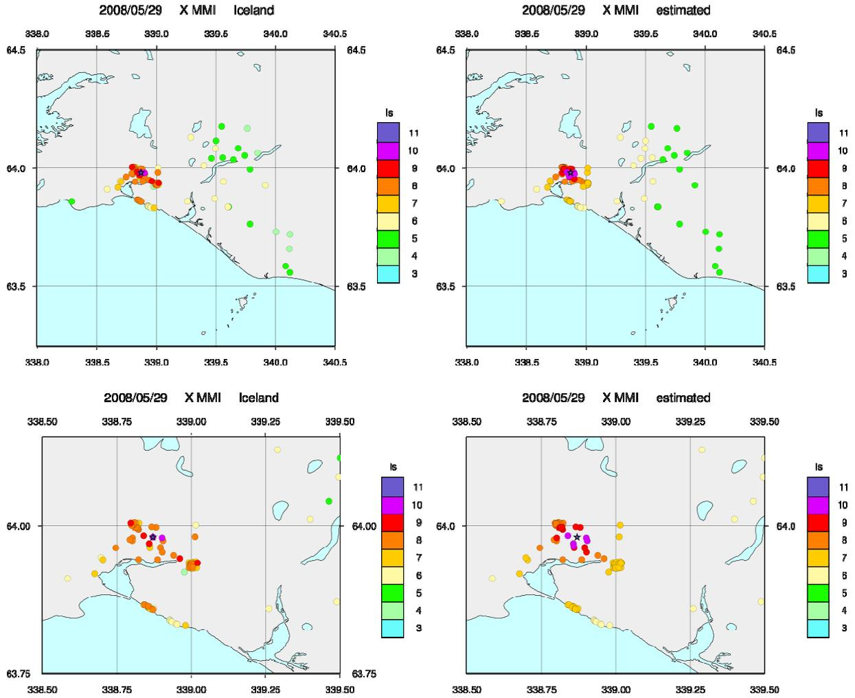
**Figure 3.3.** Macroseismic field of the 2008/05/29 earthquake in SISZ: observed intensities on the left, estimated intensities on the right. The bottom row provides a zoom of the area nearest to the epicentre. Stars denote the epicentre.
