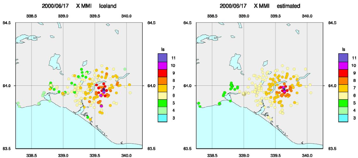
**Figure 3.2.** Macroseismic field of the 2000/06/17 earthquake in SISZ: observed intensities on the left, estimated intensities on the right. Stars denote the epicentre.
