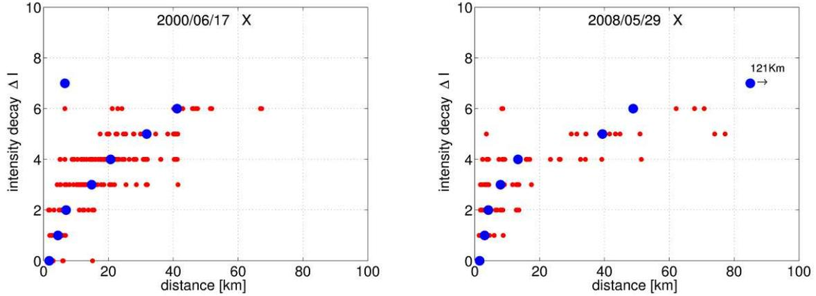
**Figure 3.1.** Intensity decay (red dots) vs. epicentral distance for the 2000/06/17 (left) and the 2008/05/29 (right) earthquakes. Blue dots denote the median of the distance subsets.
